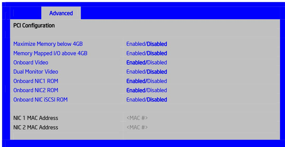
**Figure 28. Setup Utility — PCI Configuration Screen Display**
