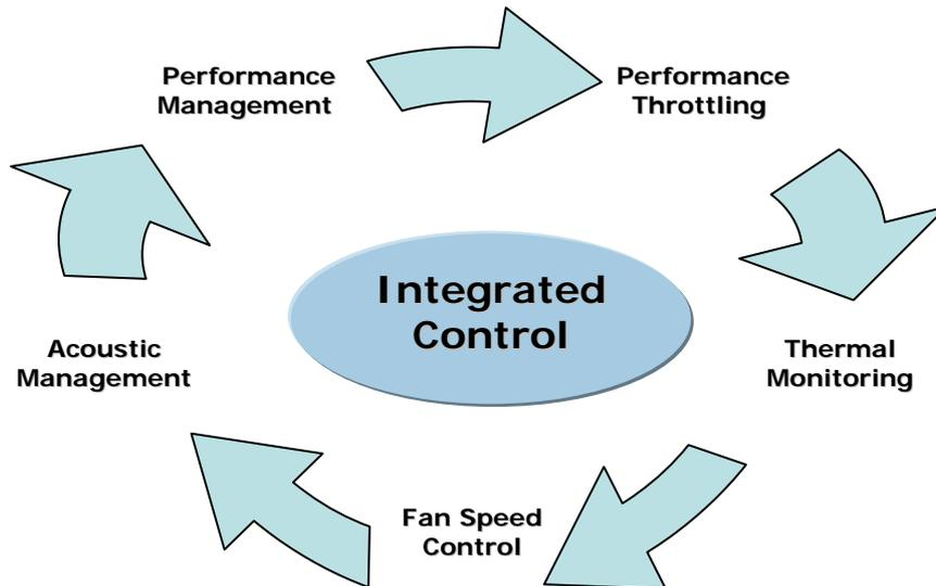
Platform control optimizes system performance and acoustics levels through:
