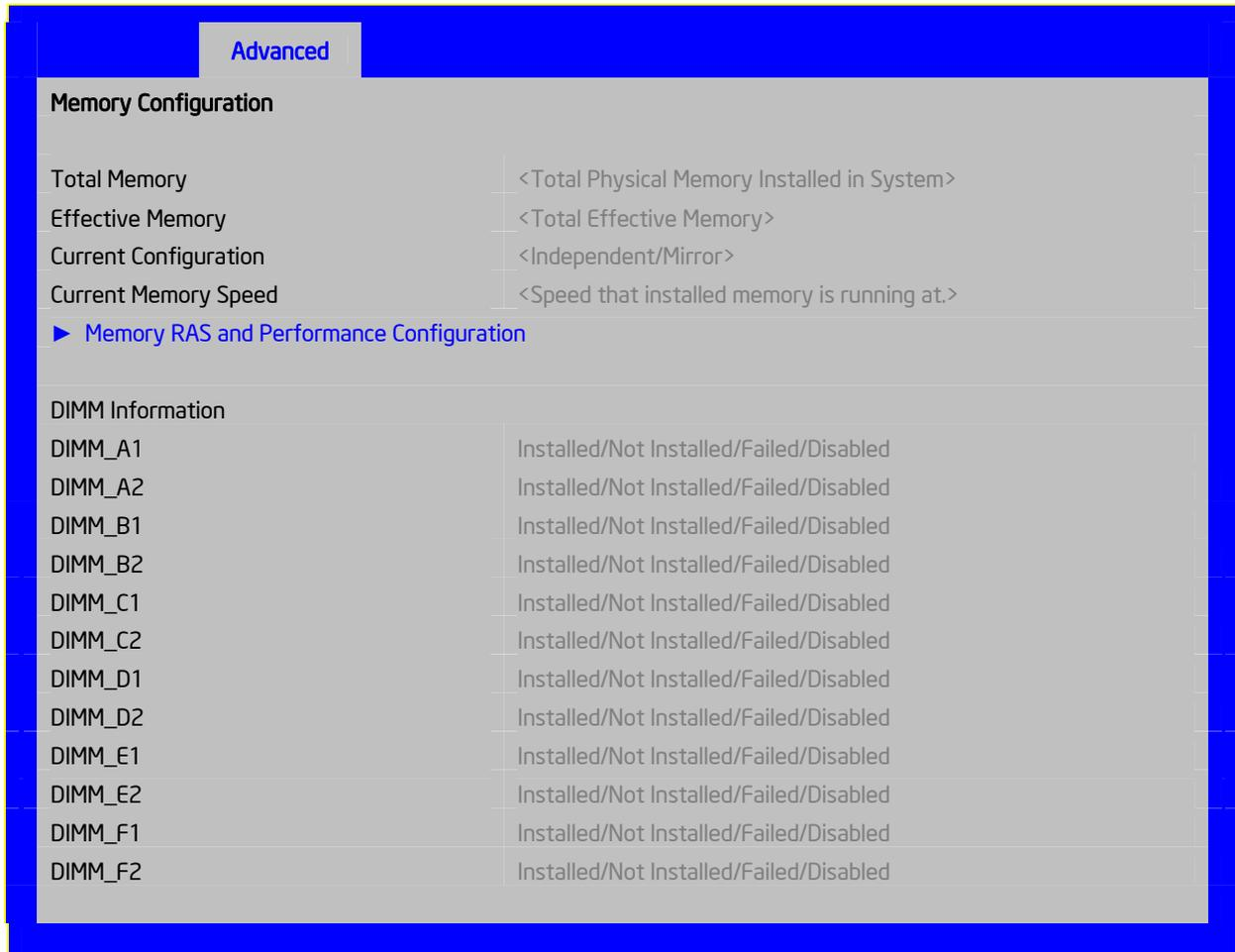
Figure 23. Setup Utility — Memory Configuration Screen Display
