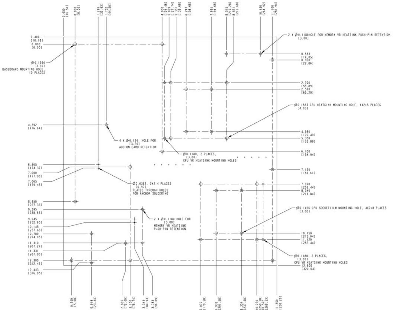
Figure 4. Intel® Workstation Board S5520SC – Mounting Hole Positions
