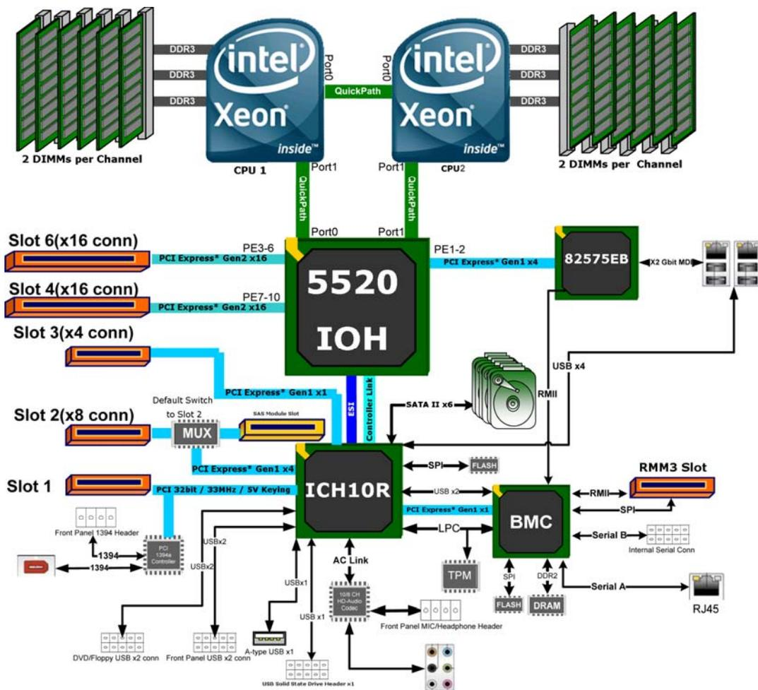
Figure 13. Intel® Workstation Board S5520SC Functional Block Diagram
