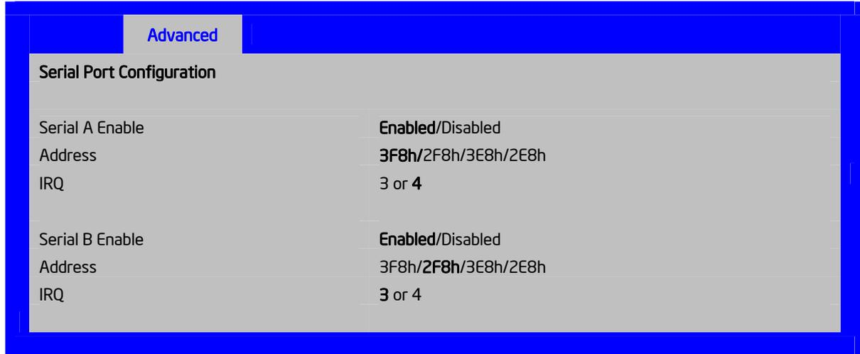
Figure 26. Setup Utility — Serial Port Configuration Screen Display
