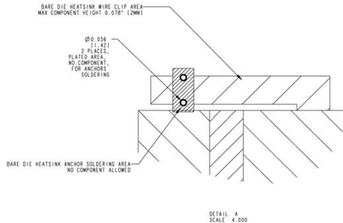
Figure 8. Intel® Workstation Board S5520SC – Primary Side Keepout Zone (2 of 2)
