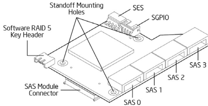
Figure 16. Intel® SAS Entry RAID Module AXX4SASMOD Component and Connector Layout
