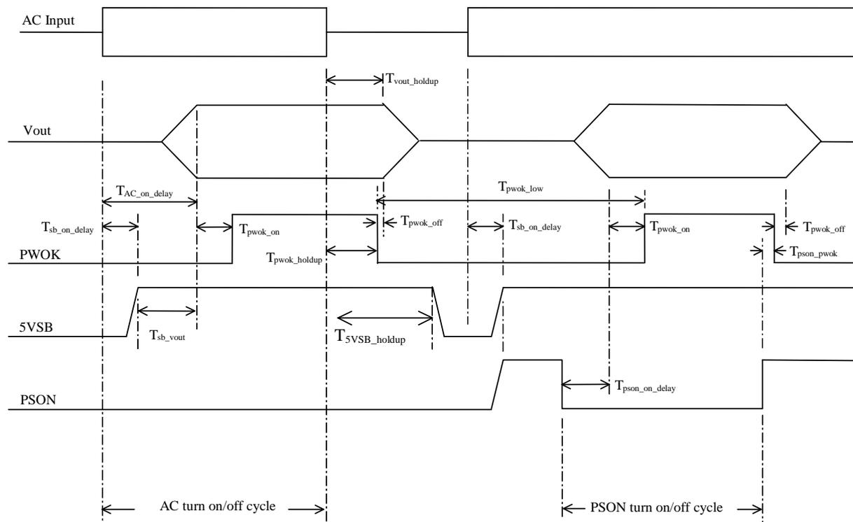
Figure 53. Turn On/Off Timing (Power Supply Signals)
