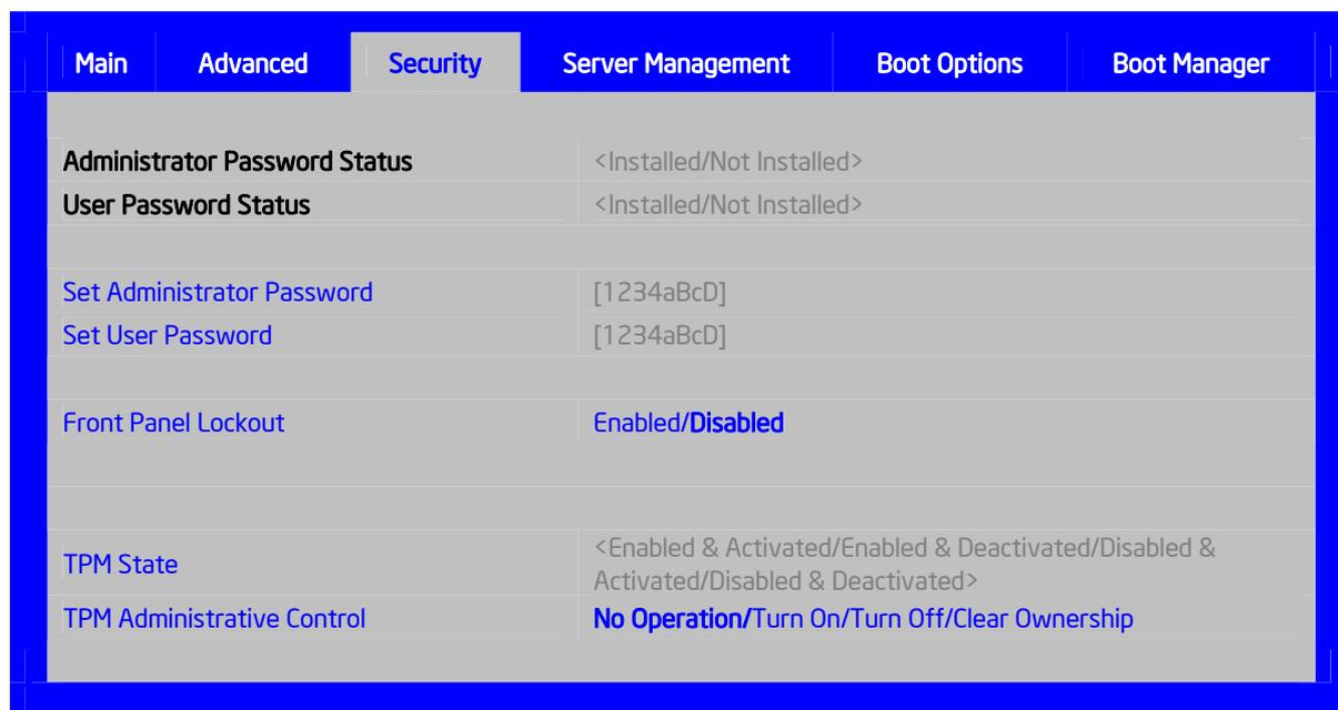
Figure 18. Setup Utility – TPM Configuration Screen
