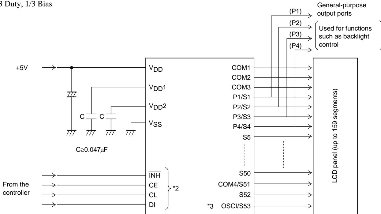
\*2 The pins to be connected to the controller (CE, CL, DI,  $\overline{\text{INH}}$ ) can handle 3.3 V or 5 V.
