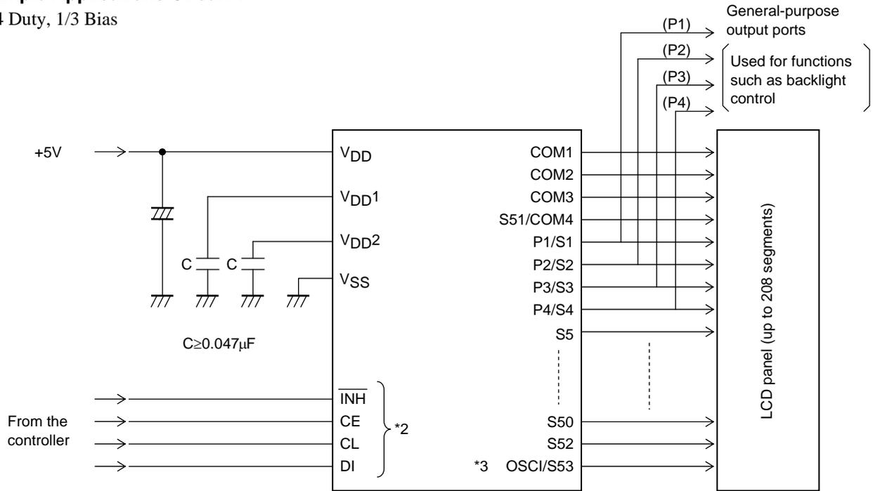
\*2 The pins to be connected to the controller (CE, CL, DI,  $\overline{\text{INH}}$ ) can handle 3.3 V or 5 V.
