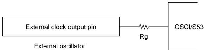
Note: Allowable current value at external clock output pin  $> \frac{V_{DD}}{R_g}$
