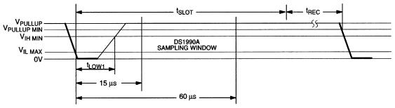
$\begin{array}{l} 60 \ \mu s \leq t_{SLOT} < 120 \ \mu s \\ 1 \ \mu s \leq \ t_{LOW1} < 15 \ \mu s \\ 1 \ \mu s \leq \ t_{REC} < \infty \end{array}$
