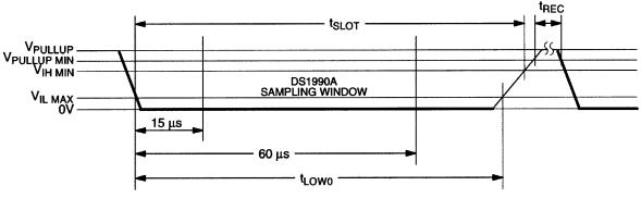
$\begin{array}{l} 60 \ \mu s \leq t_{LOW0} < t_{SLOT} < 120 \ \mu s \\ 1 \ \mu s \leq t_{REC} < \infty \end{array}$
