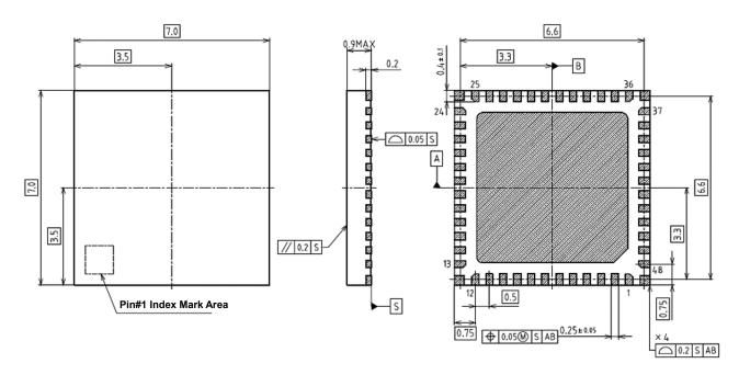
Backside heatsink: 5.4 mm × 5.4 mm
