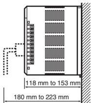
**Note:** When using Expansion Racks, the total length of the I/O Connecting Cables must be less than 12 m. When bending an I/O Connecting Cables, provide at least the minimum bending radius shown in the following diagrams.
