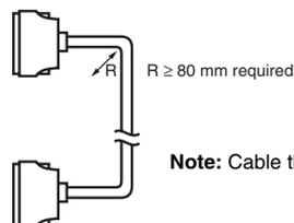
**Note:** Cable thickness: 10 mm dia.
