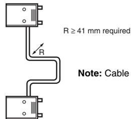
**Note:** Cable thickness: 5.1 mm dia.
