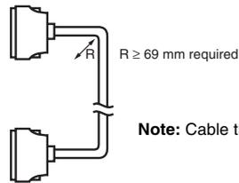
**Note:** Cable thickness: 8.6 mm dia.
