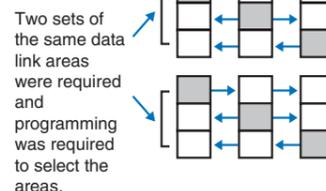
Just create the data links for one Controller Link Unit to eliminate wasted data memory. The Duplex Controller Link Units share the data links.
