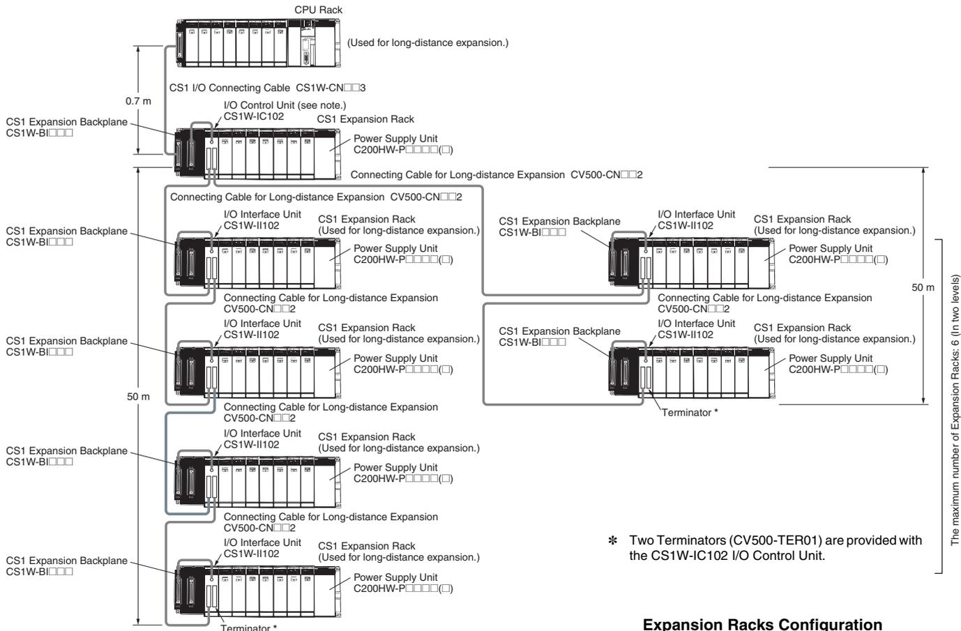
\* Two Terminators (CV500-TER01) are provided with the CS1W-IC102 I/O Control Unit.
