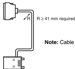
**Note:** Cable thickness: 5.1 mm dia.
