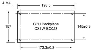
Note: An Expansion Backplane cannot be connected to a 2-slot CPU Backplane.
