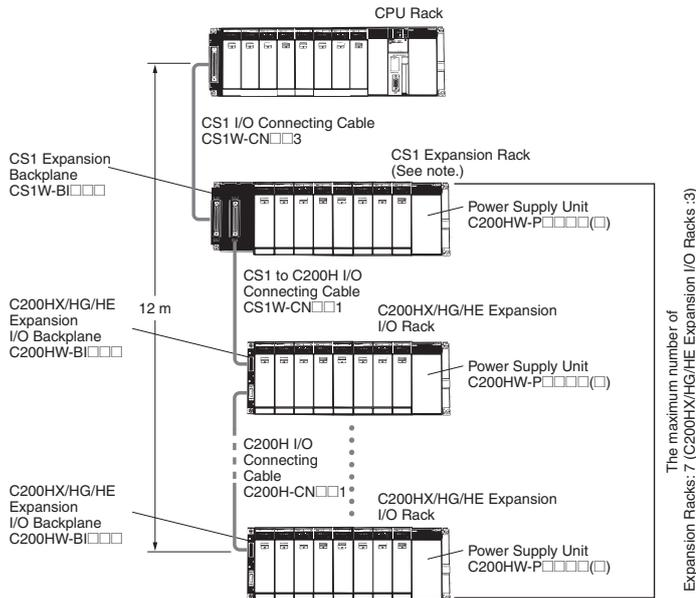
**Note:** Multiple CS1 Expansion Racks can be connected, but the total number of Expansion Racks must not exceed the maximum of 7. In addition, the Racks must be connected in order, with CS1 Expansion Racks connected before C200HX/HG/HE Expansion I/O Racks.
