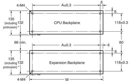
\* The CS1D Backplane has no protrusions.
