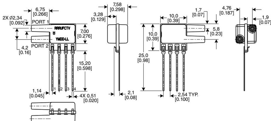
**SIP HH:** Fastener mount dual radial barbed ports, same side
