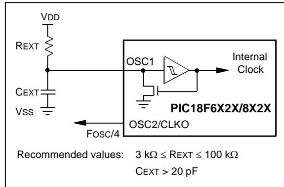
The RCIO Oscillator mode functions like the RC mode except that the OSC2 pin becomes an additional general purpose I/O pin. The I/O pin becomes bit 6 of PORTA (RA6).
