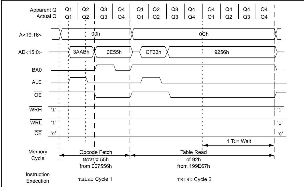
**FIGURE 6-5: EXTERNAL MEMORY BUS TIMING FOR TBLRD (EXTENDED MICROCONTROLLER MODE)**
