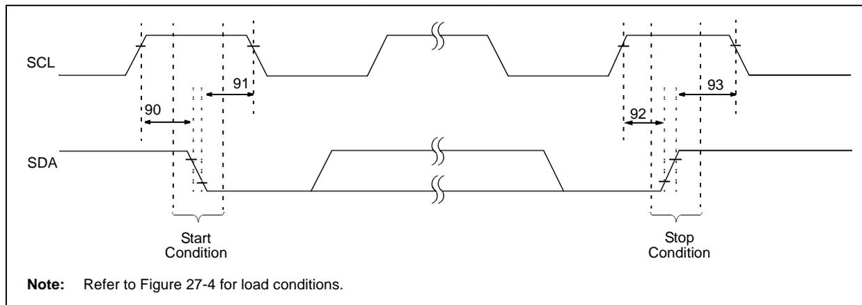
**TABLE 27-19: I<sup>2</sup>C™ BUS START/STOP BITS REQUIREMENTS (SLAVE MODE)**
