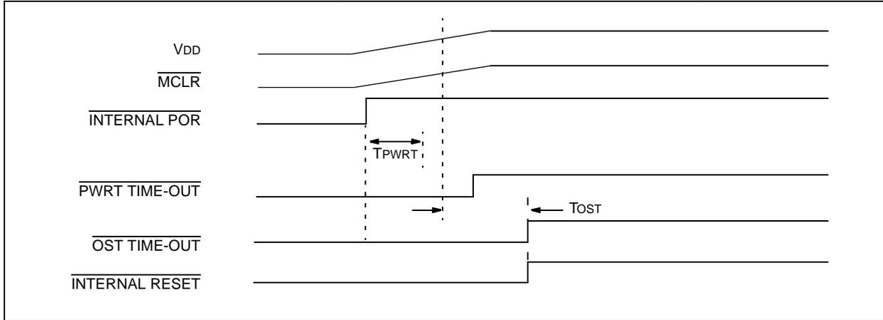
**FIGURE 3-7: TIME-OUT SEQUENCE ON POR W/PLL ENABLED ( $\overline{\text{MCLR}}$  TIED TO  $V_{DD}$  VIA 1 k $\Omega$  RESISTOR)**
