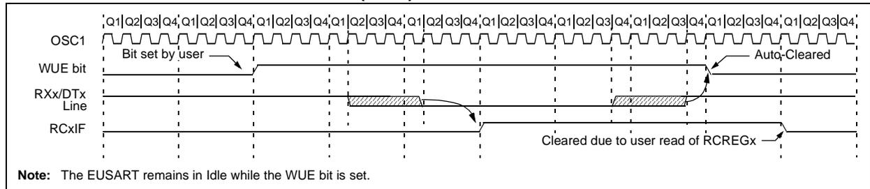
**FIGURE 19-8: AUTO-WAKE-UP BIT (WUE) TIMINGS DURING SLEEP**
