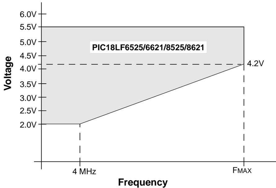
For PIC18F6525/6621 and PIC18F8525/8621 in Microcontroller mode:
