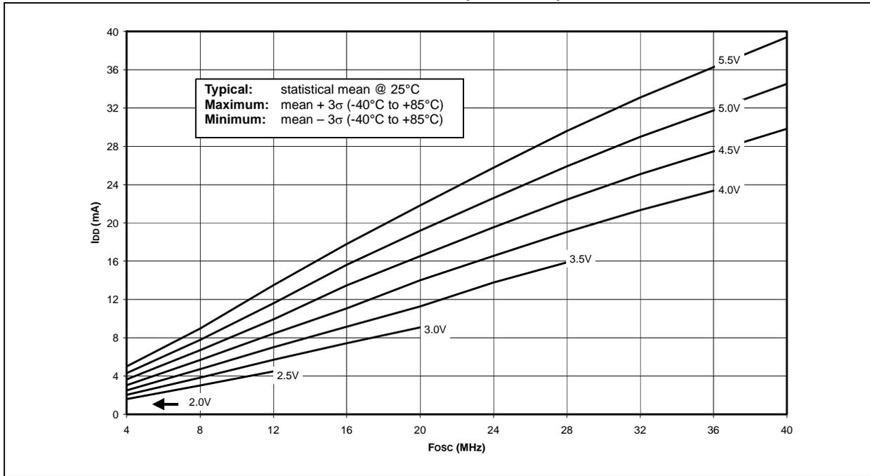
**FIGURE 28-2: MAXIMUM I<sub>DD</sub> vs. F<sub>osc</sub> OVER V<sub>DD</sub> (HS MODE)**
