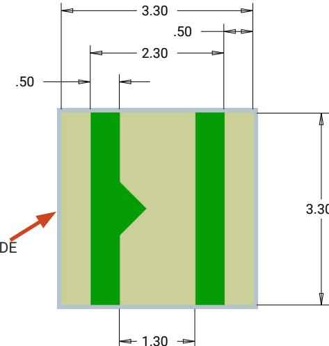
**Alternate Bottom View**
