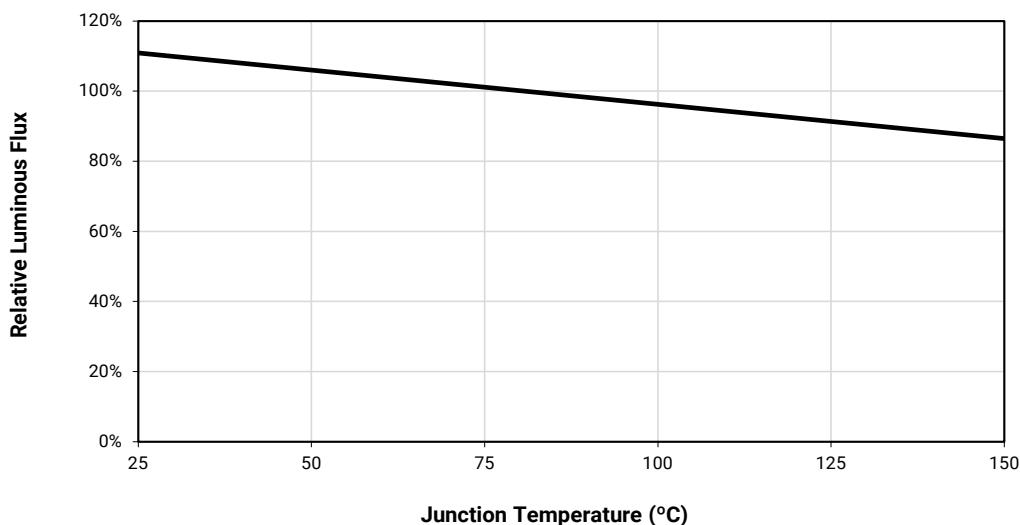
**RELATIVE RADIANT FLUX VS. JUNCTION TEMPERATURE - ROYAL BLUE ( $I_F = 350 \text{ mA}$ )**
