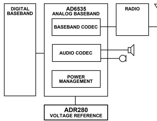
Figure 21. GSM Mobile Station Application
