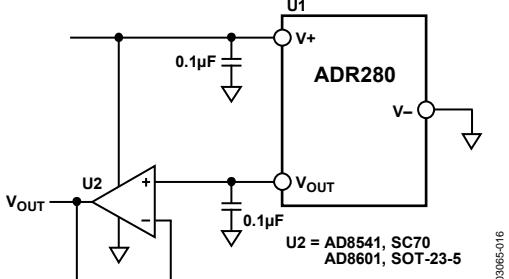
Figure 14. Buffered Output
