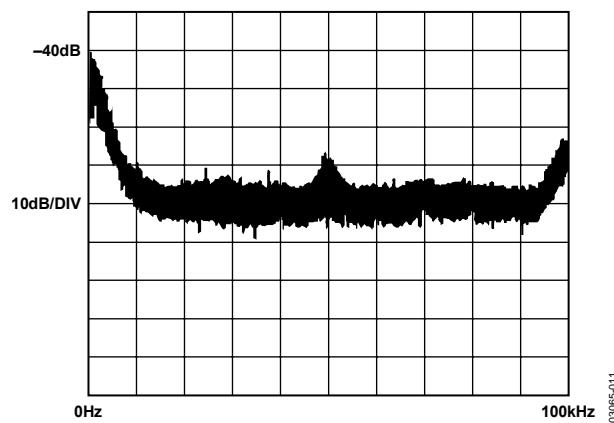
Figure 9. Voltage Noise Density, 0 Hz to 100 kHz
