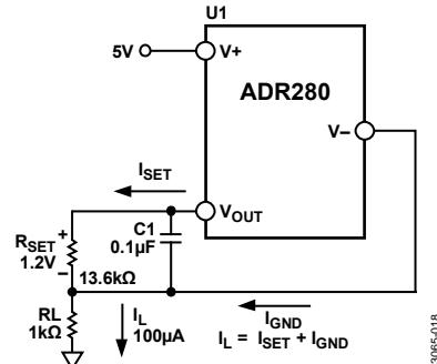
Figure 16. Low Cost Current Source
