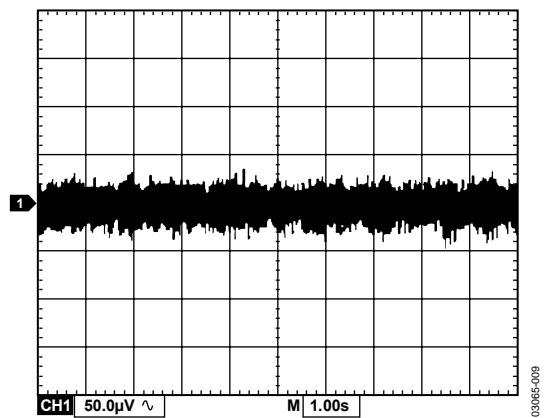
Figure 7. Noise Voltage Peak-to-Peak, 10 Hz to 10 kHz
