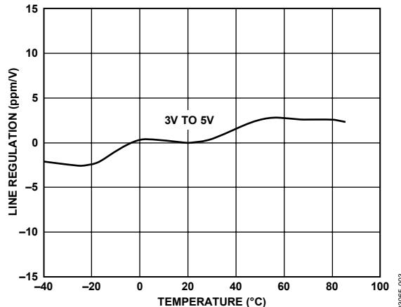
Figure 3. Line Regulation vs. Temperature
