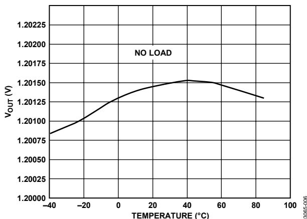
Figure 4.  $V_{OUT}$  vs. Temperature
