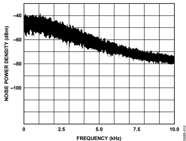
Figure 8. Output Noise Density Plot ( $V_+ = 3.6\text{ V}$ ,  $C_{\text{OUT}} = 1\text{ }\mu\text{F}$ ,  $C_{\text{IN}} = 1\text{ }\mu\text{F}$ )
