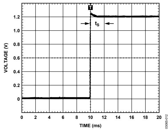
Figure 10. Settling Time
