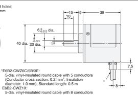
5-dia. vinyl-insulated round cable with 8 conductors (Conductor cross section: 0.2 mm², Insulation diameter: 1.0 mm), Standard length: 0.5 m
