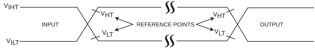
FIGURE 8-5: AC INPUT/OUTPUT REFERENCE WAVEFORMS
