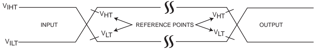
FIGURE 8-5: AC INPUT/OUTPUT REFERENCE WAVEFORMS
