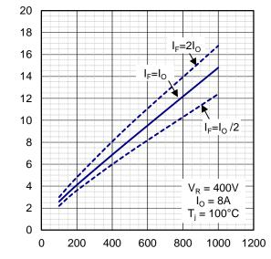
RATE OF CHANGE OF CURRENT :  $-di/dt(A/\mu s)$   $di/dt-I_{Rp}$  CHARACTERISTICS
