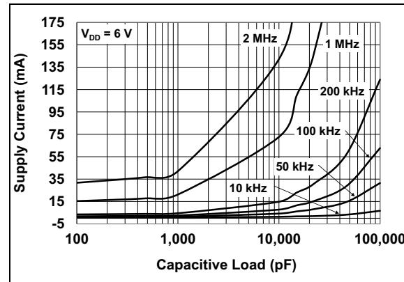
FIGURE 2-18: Supply Current vs. Capacitive Load ( $V_{DD} = 6\text{V}$ ).
