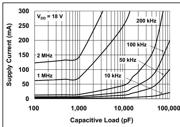
FIGURE 2-16: Supply Current vs. Capacitive Load ( $V_{DD} = 18\text{V}$ ).
