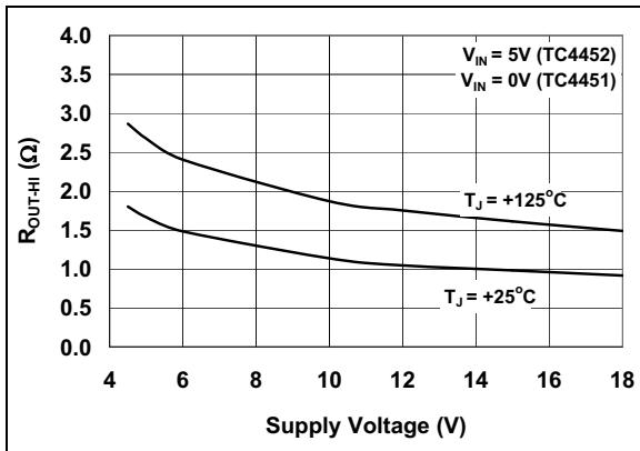
FIGURE 2-14: High-State Output Resistance vs. Supply Voltage.
