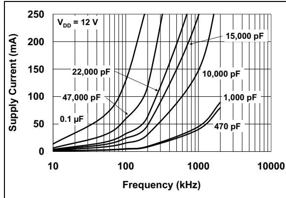
**FIGURE 2-20:** Supply Current vs. Frequency ( $V_{DD} = 12\text{V}$ ).
