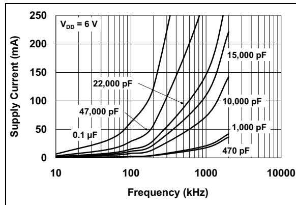
**FIGURE 2-21:** Supply Current vs. Frequency ( $V_{DD} = 6\text{V}$ ).
