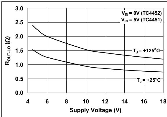
FIGURE 2-15: Low-State Output Resistance vs. Supply Voltage.
