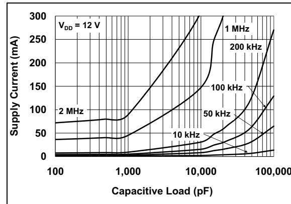
FIGURE 2-17: Supply Current vs. Capacitive Load ( $V_{DD} = 12\text{V}$ ).
