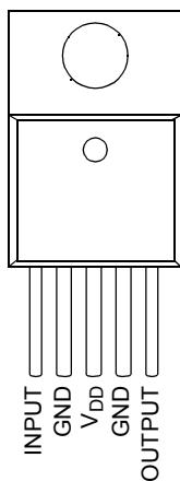
**Note 1:** Duplicate pins must both be connected for proper operation.
