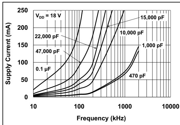
**FIGURE 2-19:** Supply Current vs. Frequency ( $V_{DD} = 18\text{V}$ ).
