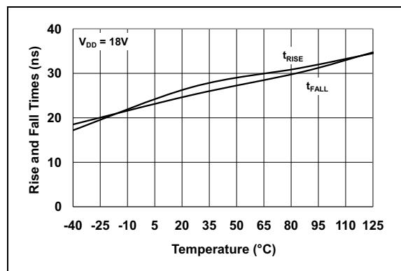
**FIGURE 2-5:** Rise and Fall Times vs. Temperature.
