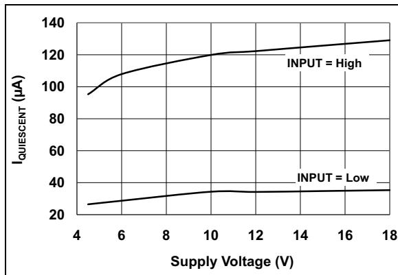
**FIGURE 2-10:** Quiescent Supply Current vs. Supply Voltage.
