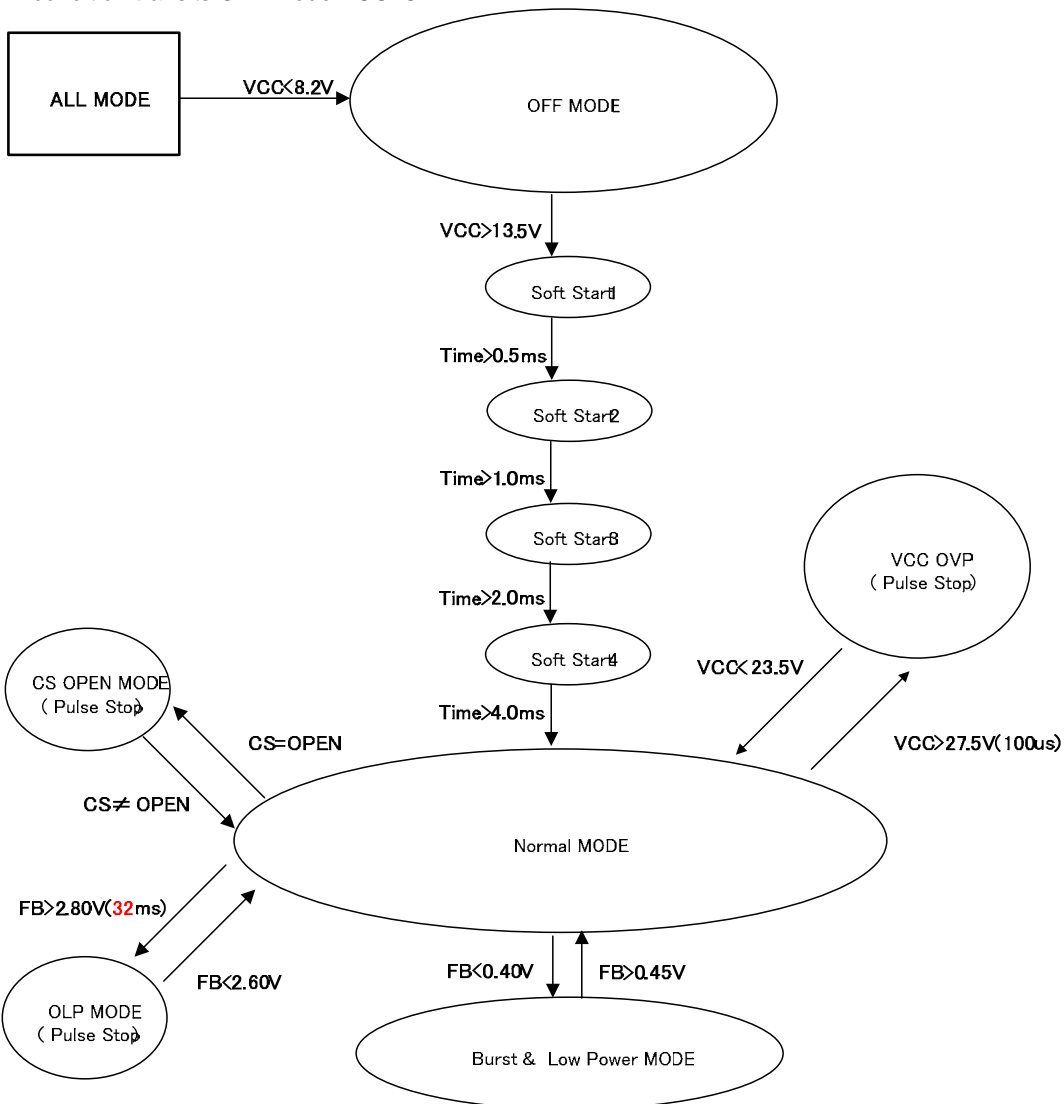
Figure 18. The sequence diagram (BM1PXX1 Series)
