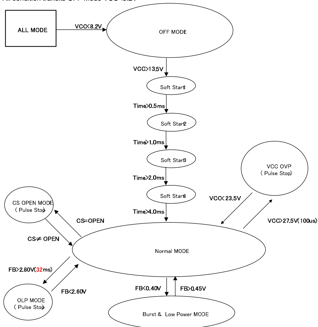
Figure 18. The sequence diagram (BM1PXX1 Series)
