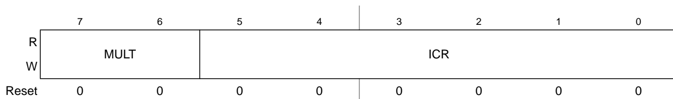
Figure 10-4. IIC Frequency Divider Register (IICF)
