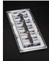
HB-IP-2X6-W D: 173 x 71,4 mm H: 11,4 mm Typ. FWHM: 58° Typ. eff: 94% PMMA LEDs: 12
