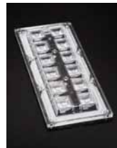
HB-IP-2X6-W D: 173 x 71,4 mm H: 11,4 mm Typ. FWHM: 58° Typ. eff: 94% PMMA LEDs: 12
