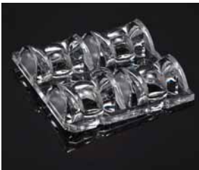
HB-2X2-O D: 50 x 50 mm H: 10,6 mm PMMA Typ. eff: 94% LEDs: 4 Oval beam type suitable for warehouse aisle lighting
