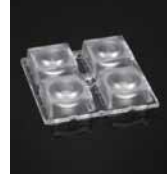
HB-2X2-RW D: 50x50 mm H: 8,5 mm PMMA Typ. FWHM: 51° Typ. eff: 89% LEDs: 4
