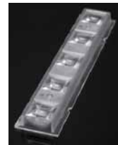
HB-5X1-FLAT-W D: 123 x 25 mm H: 8,5 mm PMMA Typ. FWHM: 54° Typ. eff: 91% LEDs: 5
