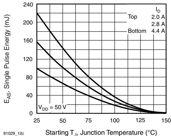
Fig. 12c - Maximum Avalanche Energy vs. Drain Current
