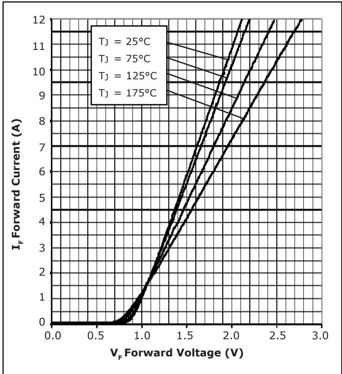
Figure 1. Forward Characteristics
