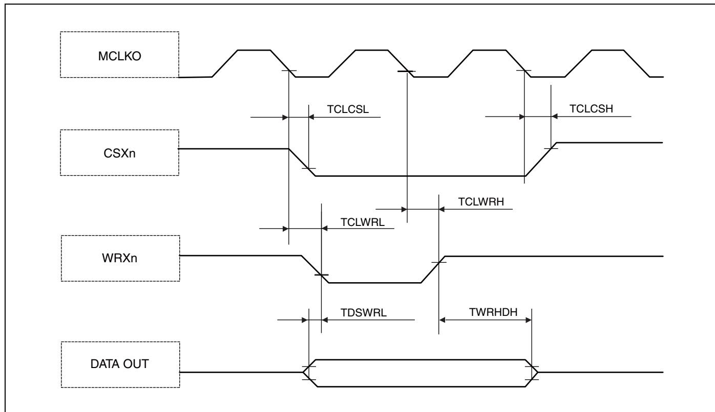
*Asynchronous Write Access - Byte Control Type*
