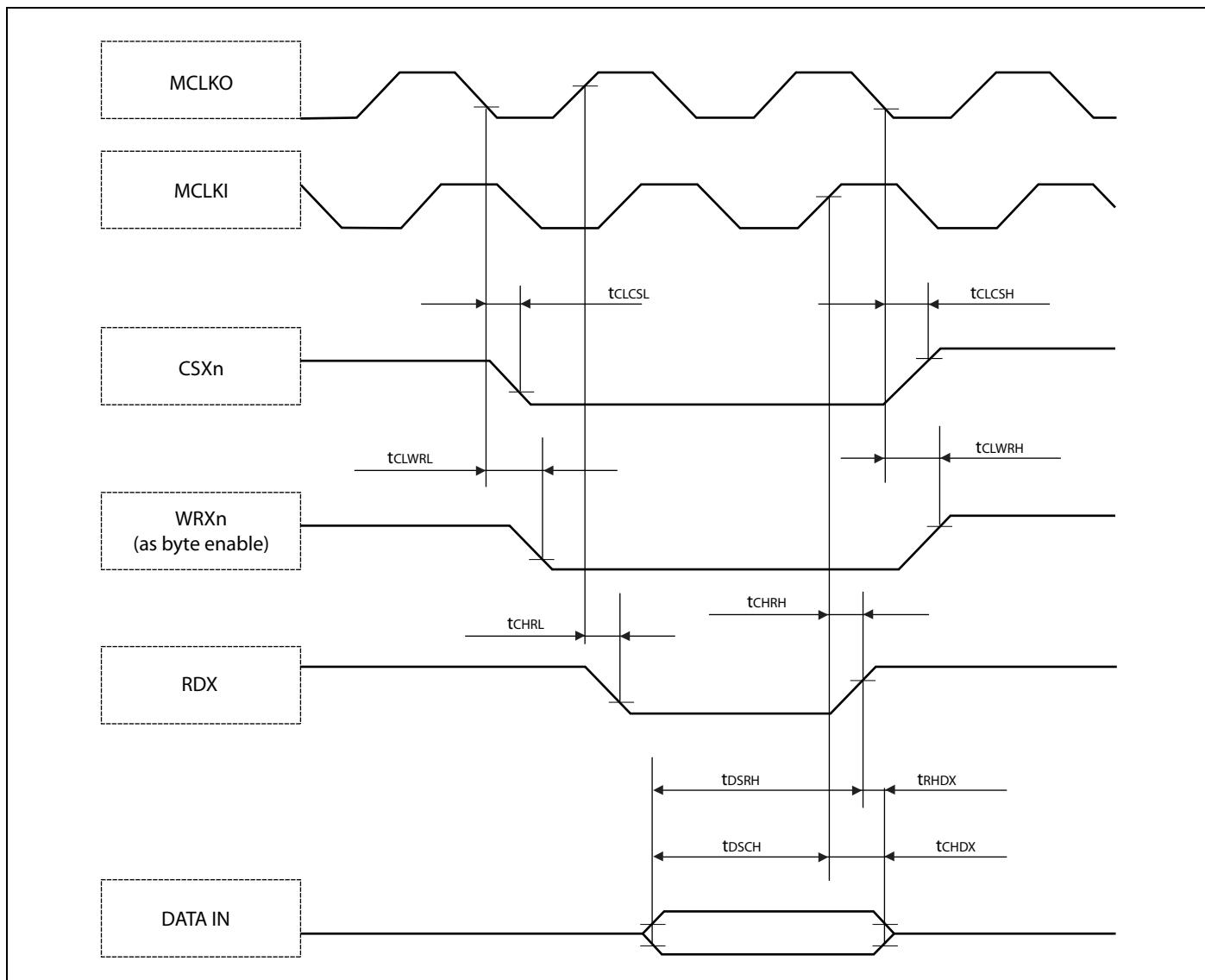
*Synchronous/Asynchronous Read Access with Internal MCLKO --> MCLKI Feedback*
