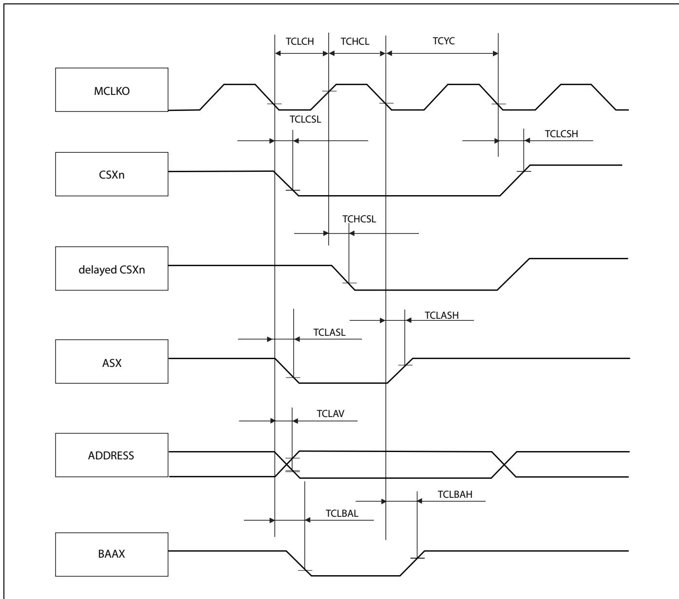
*Synchronous/Asynchronous Read Access With External MclkI Input*
