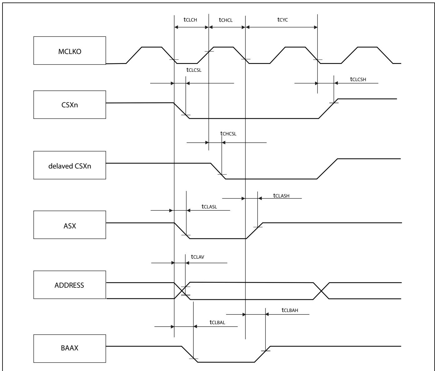
*Synchronous/Asynchronous Read Access With External MclkI Input*
