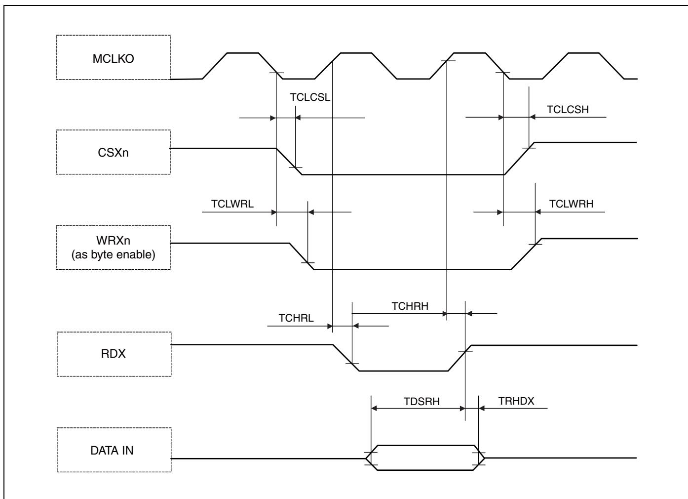
*Synchronous Write Access - Byte Control Type*
