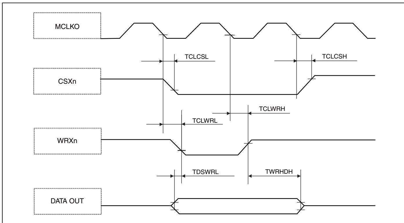
**Asynchronous Write Access - Byte Control Type**
