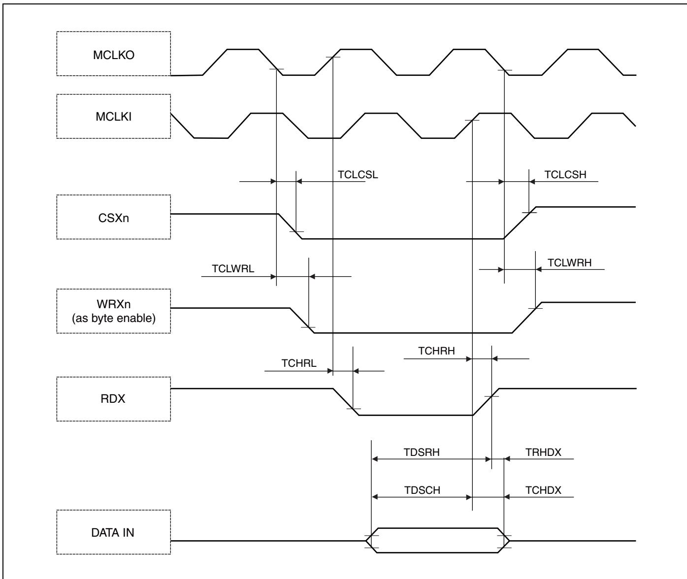
*Synchronous/Asynchronous Read Access with Internal MCLKO --> MCLKI Feedback*
