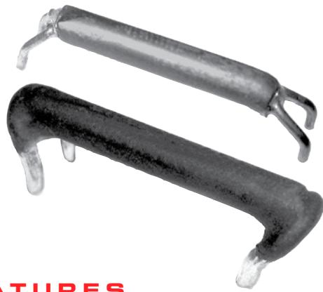
Ohmite's Four Terminal Bare Element Resistors provide ultra low resistance values (to  $0.0005\Omega$ ) for relatively high current requirements, with the advantages of a Kelvin configuration and PC Board mounting capability.
