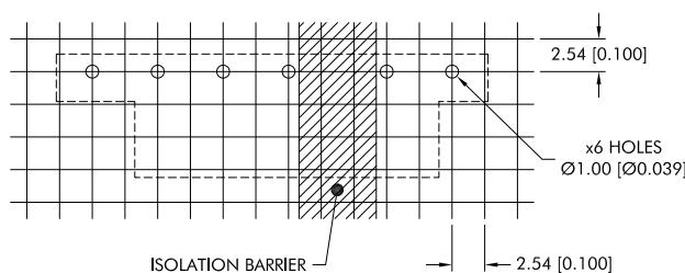
The isolation barrier shown must not have any copper traces even on internal layers. This is to avoid compromising the creepage and clearance distance. PCB layouts must take into consideration the required clearance and creepage requirements to maintain the clearance and creepage of the isolation barrier. All dimensions in mm (inches).
