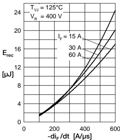
Fig. 7 Typ. recovery energy  $E_{rec}$  versus  $-di_F/dt$
