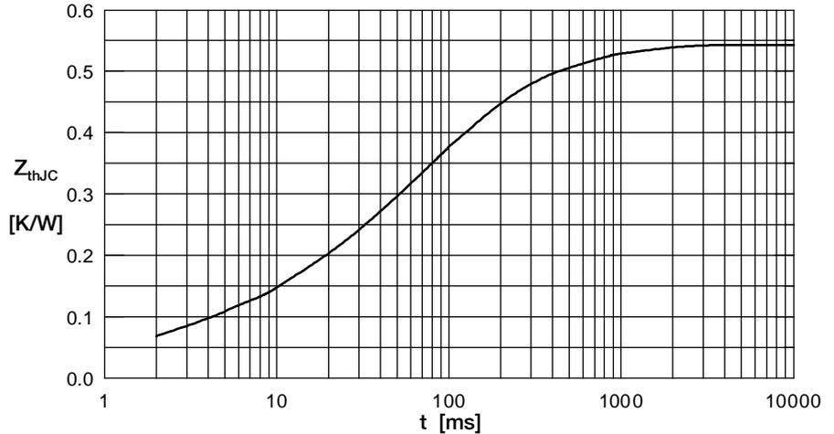
Fig. 8 Transient thermal impedance junction to case
