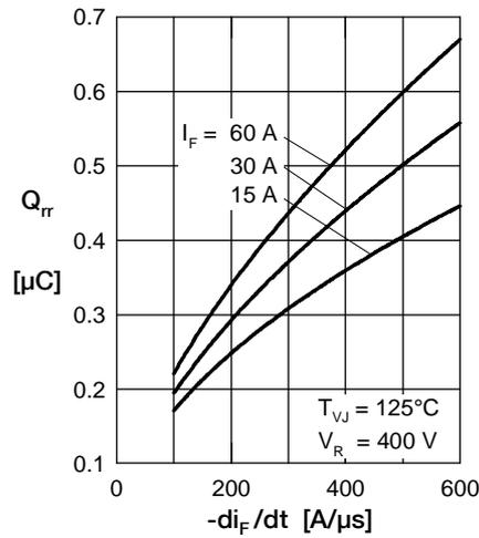
Fig. 2 Typ. reverse recov. charge  $Q_{rr}$  versus  $-di_F/dt$
