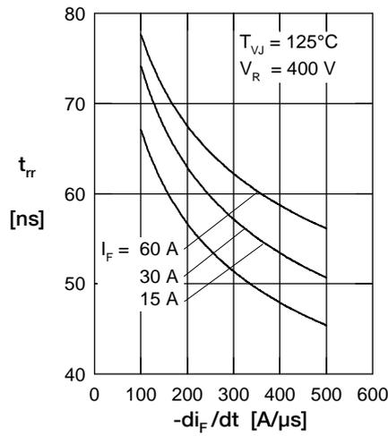
Fig. 5 Typ. reverse recov. time  $t_{tr}$  versus  $-di_F/dt$
