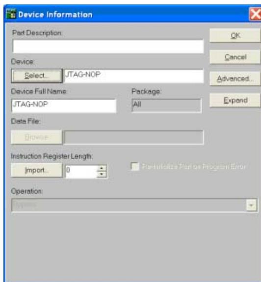
6. Double-click on the **Device Select** button. Scroll to the **ispMACH 4000** Device Family selection. Select **LC4064V(B)-32IO** for the Device and click **OK**. See Figure 35.
