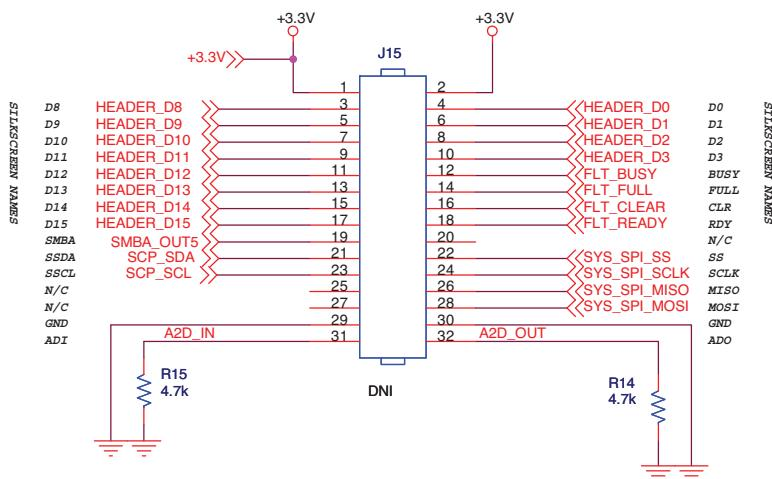
The interface has generic I/Os, SPI control signals, I<sup>2</sup>C control and fault logging signals. All of these can be set up and programmed by the user for custom I/Os.
