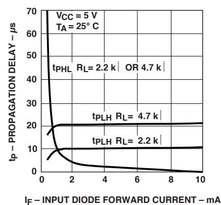
Figure 8. Propagation delay vs. input diode forward current.
