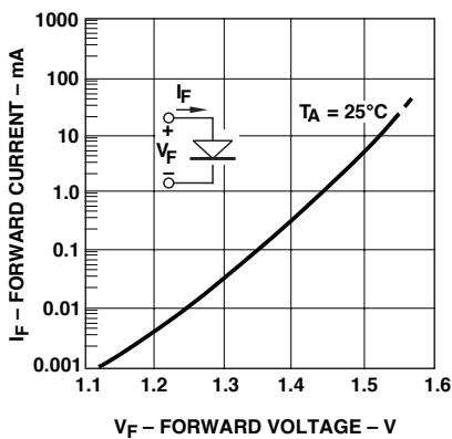
Figure 4. Input diode forward current vs. forward voltage.
