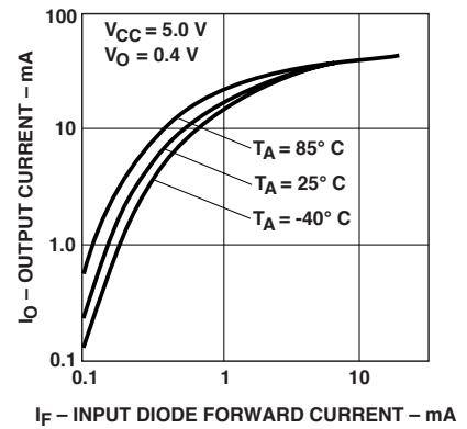
Figure 3. Output current vs. input diode forward current.
