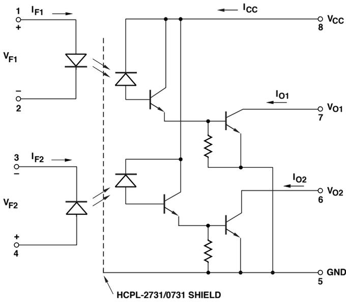
USE OF A 0.1  $\mu$ F BYPASS CAPACITOR CONNECTED BETWEEN PINS 5 AND 8 IS RECOMMENDED (SEE NOTE 8)
