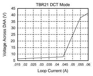
Figure 21. TBR21 Mode I/V Characteristics, DCV[1:0] = 11, MINI[1:0] = 00, ILIM = 1
