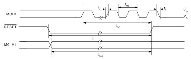
Figure 2. General Inputs Timing Diagram
