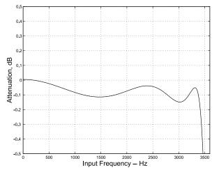
Figure 12. IIR Receive Filter Passband Ripple
