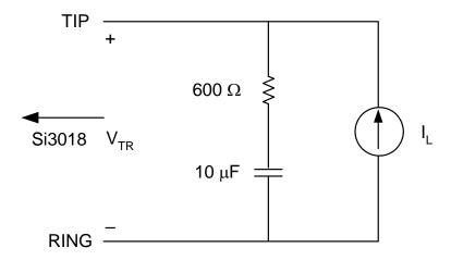
Figure 1. Test Circuit for Loop Characteristics
