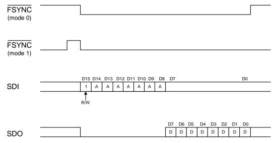
Figure 29. Secondary Communication Data Format—Read Cycle
