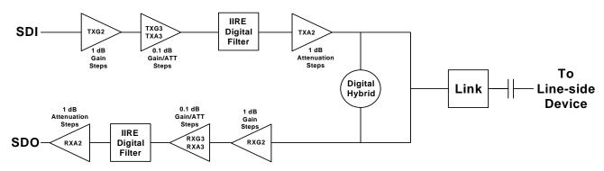
Figure 25. Si3056 Signal Flow Diagram
