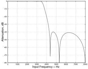
Figure 11. IIR Receive Filter Response
