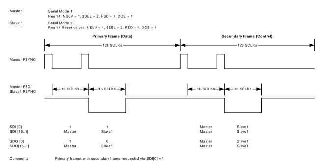
Figure 32. Daisy Chaining of a Single Slave (Frame FSD)
