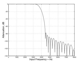
Figure 9. FIR Transmit Filter Response
