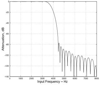
Figure 7. FIR Receive Filter Response
