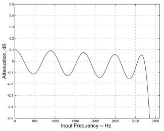
Figure 8. FIR Receive Filter Passband Ripple
