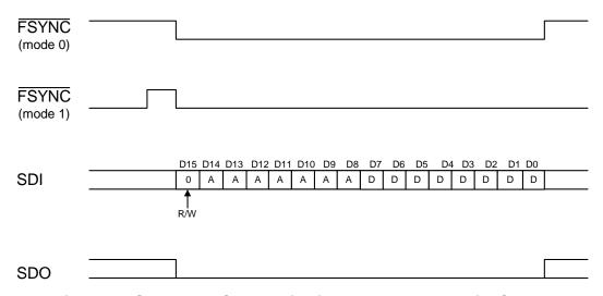
Figure 30. Secondary Communication Data Format—Write Cycle
