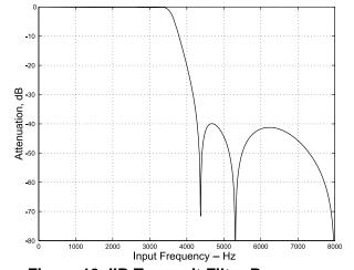
Figure 13. IIR Transmit Filter Response
