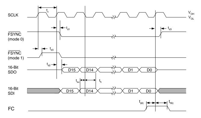
Figure 3. Serial Interface Timing Diagram (DCE = 0)
