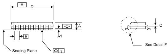
Figure 37. 16-pin Small Outline Integrated Circuit (SOIC) Package
