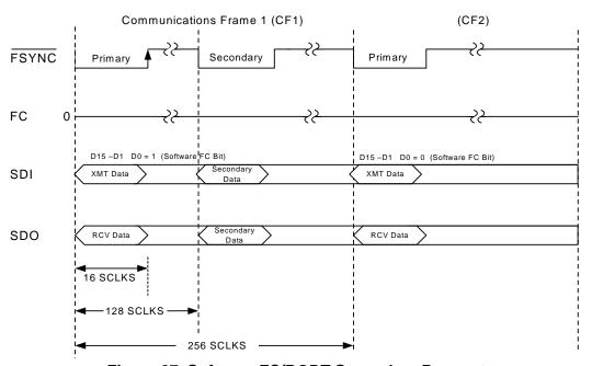
Figure 27. Software FC/RGDT Secondary Request
