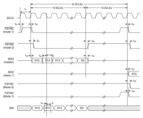
Figure 4. Serial Interface Timing Diagram (DCE = 1, FSD = 0)
