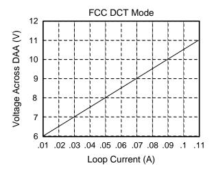
Figure 20. FCC Mode I/V Characteristics, DCV[1:0] = 11, MINI[1:0] = 00, ILIM = 0
