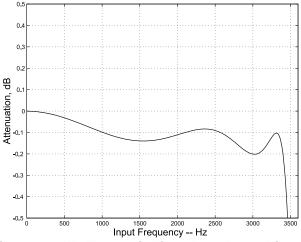
Figure 14. IIR Transmit Filter Passband Ripple
