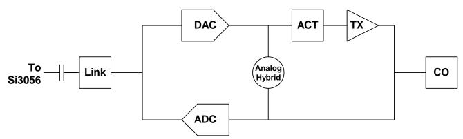
Figure 24. Line-Side Device Signal Flow Diagram
