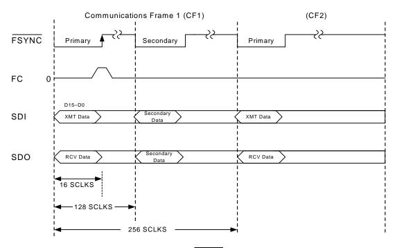
Figure 28. Hardware FC/RGDT Secondary Request
