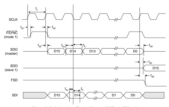
Figure 5. Serial Interface Timing Diagram (DCE = 1, FSD = 1)
