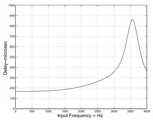
**Figure 16. IIR Transmit Group Delay**
