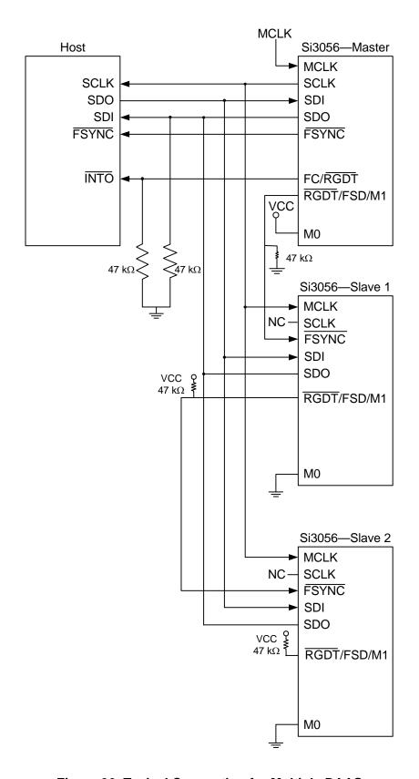
Figure 36. Typical Connection for Multiple DAAS
