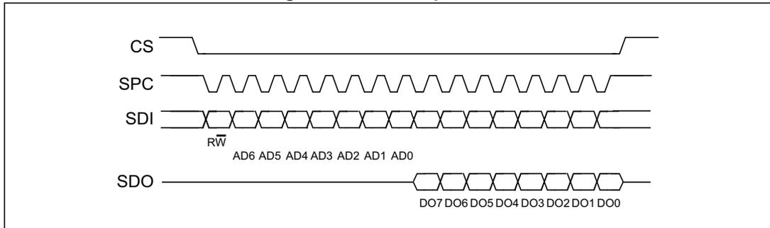
The SPI Read command is performed with 16 clock pulses. A multiple byte read command is performed by adding blocks of 8 clock pulses to the previous one.
