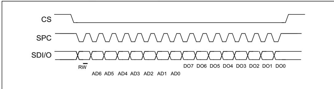
The SPI read command is performed with 16 clock pulses:
