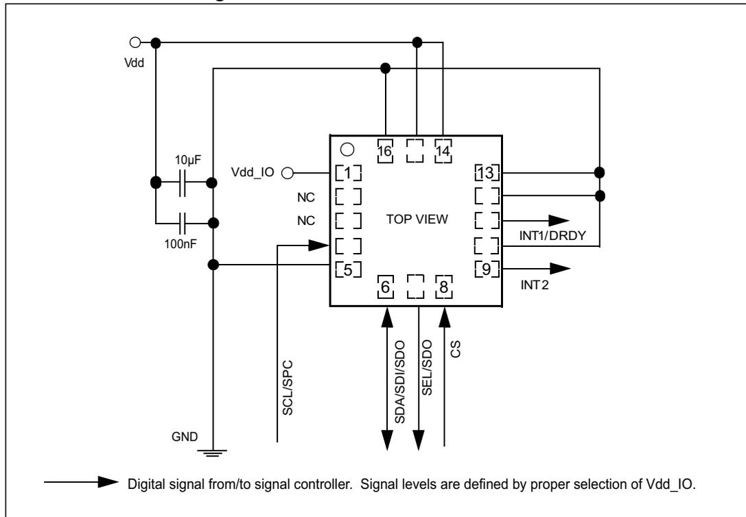
Note: Pin 15 can be connected to Vdd or GND or left unconnected.
