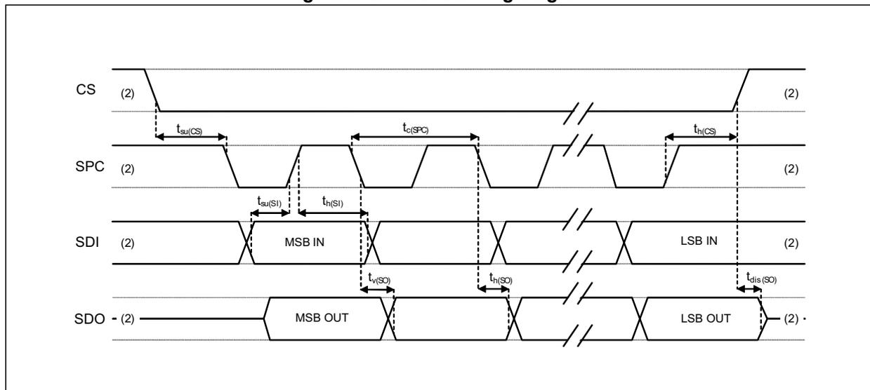
2. When no ongoing communication, data on SDO is driven by internal pull-up resistor.
