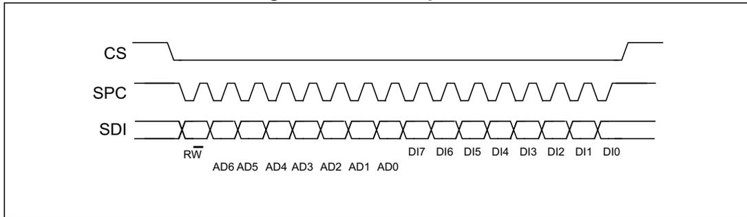
The SPI Write command is performed with 16 clock pulses. A multiple byte write command is performed by adding blocks of 8 clock pulses to the previous one.
