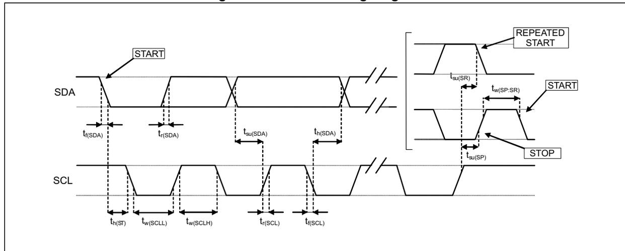
Note: Measurement points are done at 0.2·Vdd<sub>IO</sub> and 0.8·Vdd<sub>IO</sub>, for both ports.
