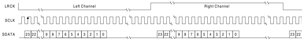
**Figure 19. I<sup>2</sup>S Serial Audio Interface**
