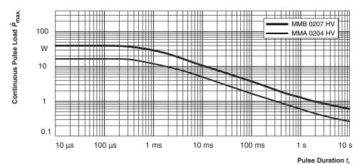
Maximum pulse load, continuous pulses; applicable if  $\bar{P} \leq P\left(\vartheta_{\rm amb}\right)$  and  $\hat{U} \leq \hat{U}_{\rm max}$ ; for permissible resistance change equivalent to 8000 h operation in power operation mode
