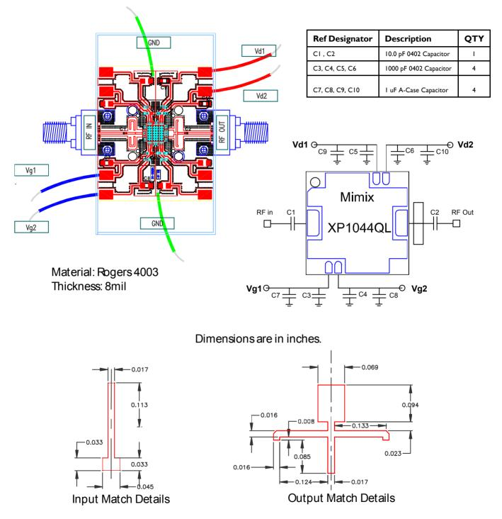
For improved performance at 6 GHz the thick transmission line (W=0.069") on the output can be extended to touch the two open stubs.
