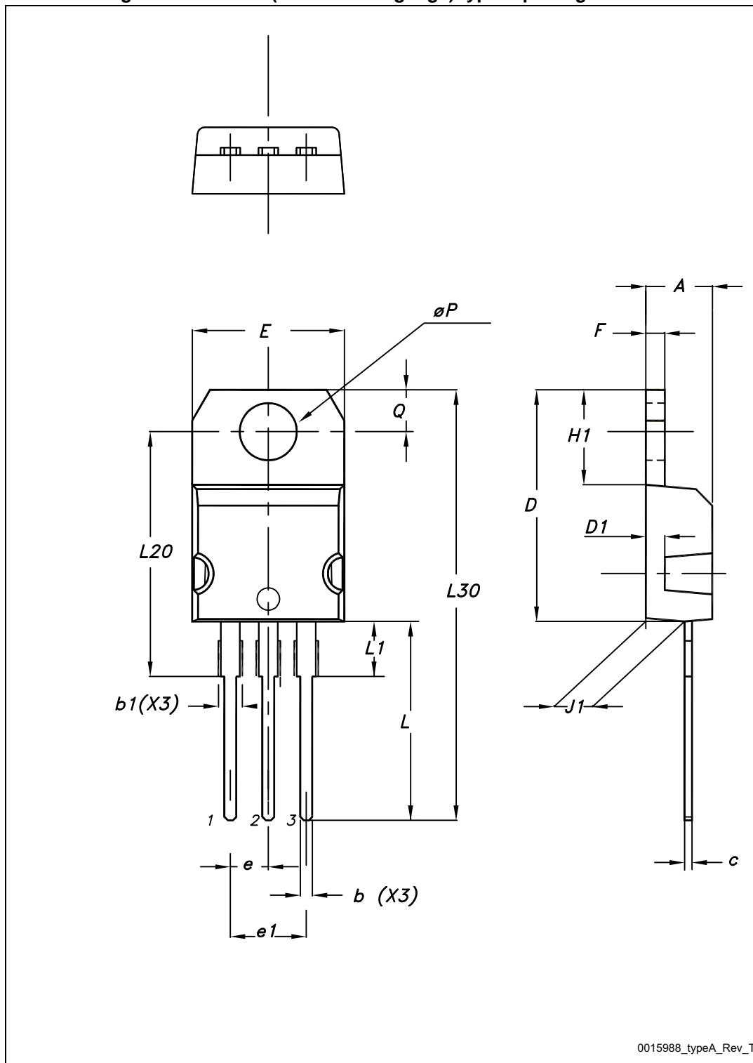
**Table 11. TO-220 (STD-ST dual gauge) type A mechanical data**
