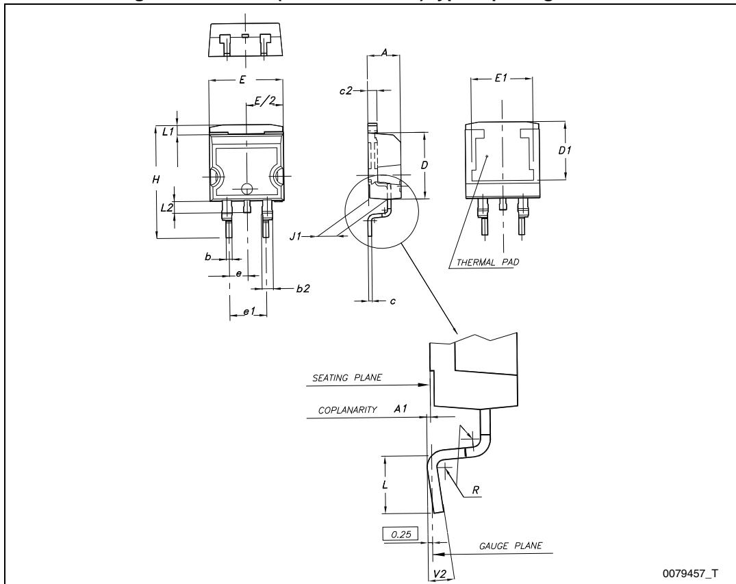
**Table 13. D<sup>2</sup>PAK (SMD 2L STD-ST) type A mechanical data**
