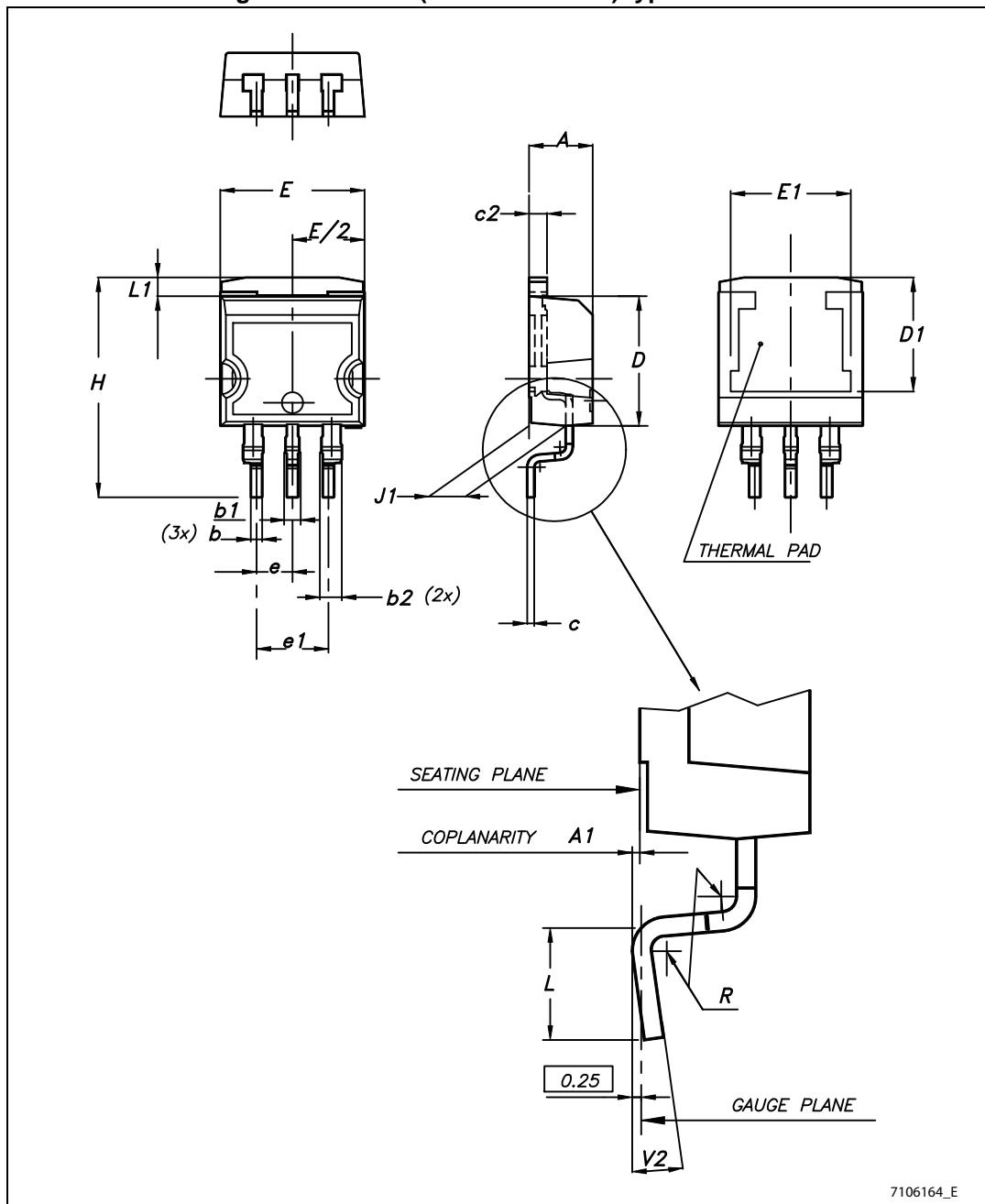
**Table 14. D<sup>2</sup>PAK (SMD 3L STD-ST) type A mechanical data**
