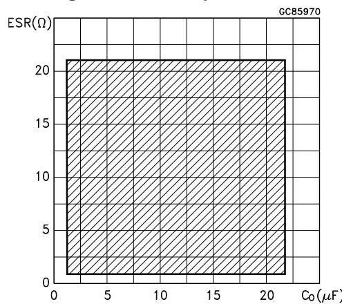
**Figure 23. Stability for 12 V**
