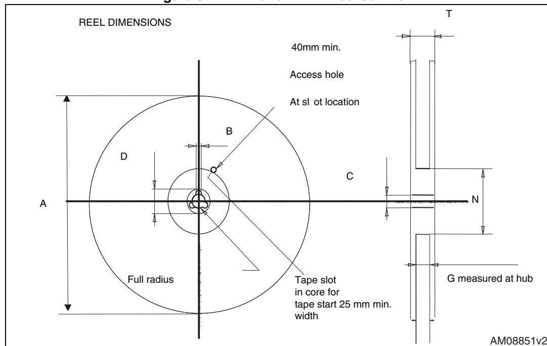
Table 15. DPAK and D<sup>2</sup>PAK tape and reel mechanical data
