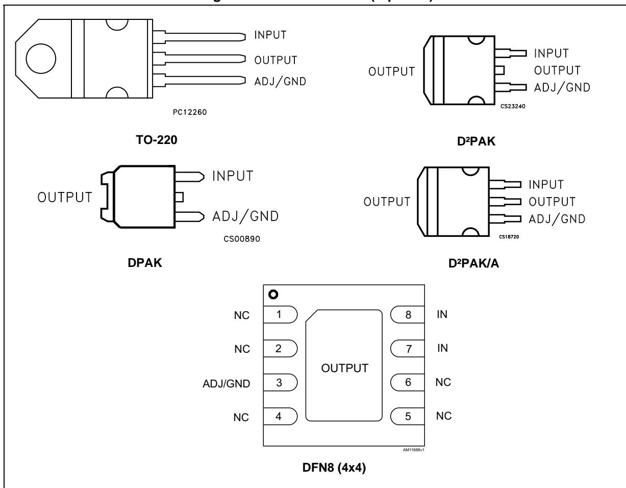
Note: The TAB is physically connected to the output (this is valid for the TO-220 package too).
