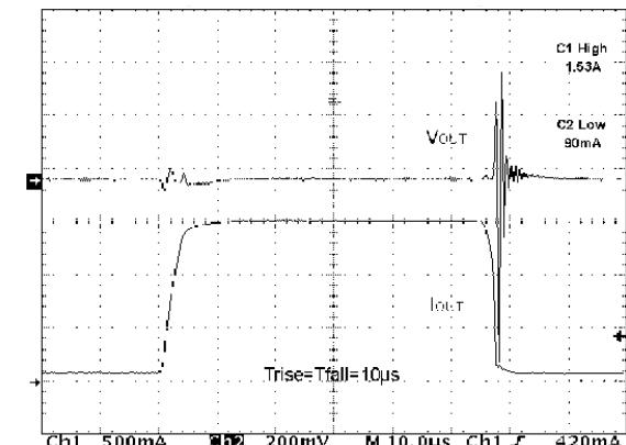
$V_I = 13 \text{ V}$ ,  $I_O = 0.1 \text{ to } 1.5 \text{ A}$ ,  $C_I = 1 \mu\text{F}$  (tant),  $C_O = 10 \mu\text{F}$  (tant),  $C_{ADJ} = 1 \mu\text{F}$
