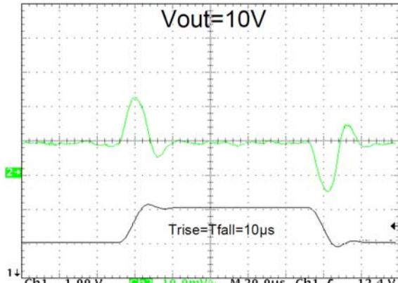
$V_I = 12$  to  $13$  V,  $I_O = 200$  mA,  $C_I = 1$   $\mu F$  (tant),  $C_O = 10$   $\mu F$  (tant), No  $C_{ADJ}$
