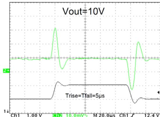
$V_I = 12$  to  $13$  V,  $I_O = 200$  mA,  $C_I = 1$   $\mu F$  (tant),  $C_O = 10$   $\mu F$  (tant), No  $C_{ADJ}$
