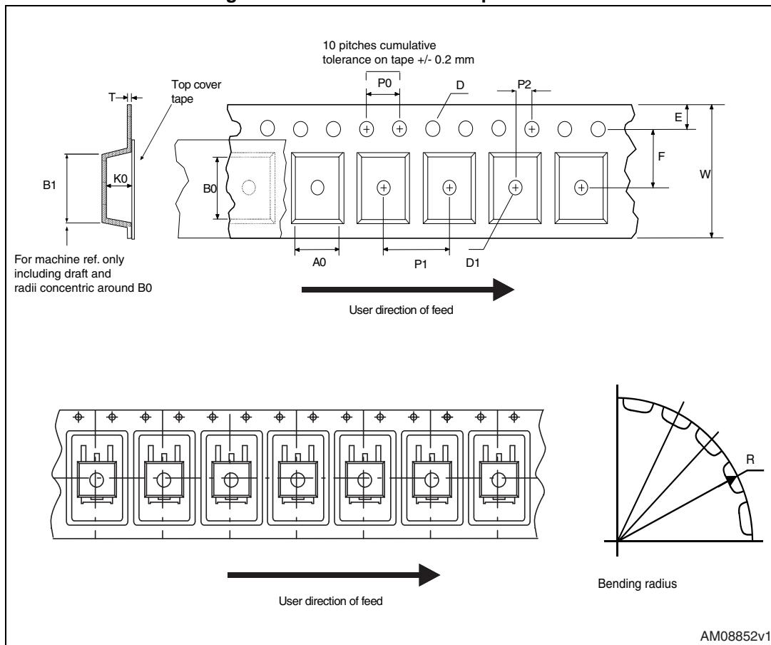
Figure 37. DPAK and D<sup>2</sup>PAK reel outline
