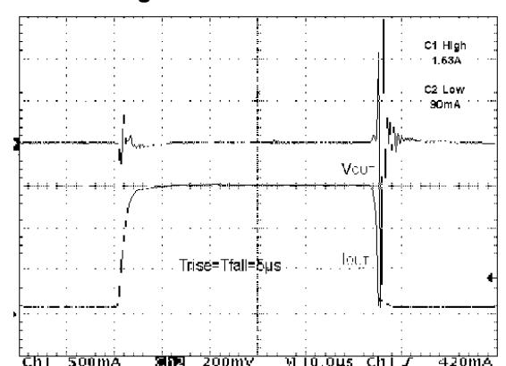
$V_I = 13$  V,  $I_O = 0.1$  to  $1.5$  A,  $C_I = 1$   $\mu F$  (tant),  $C_O = 10$   $\mu F$  (tant),  $C_{ADJ} = 1$   $\mu F$
