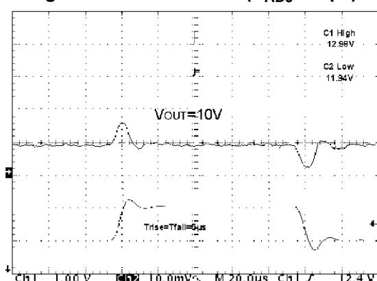
$V_I = 12$  to  $13$  V,  $I_O = 200$  mA,  $C_I = 1$   $\mu F$  (tant),  $C_O = 10$   $\mu F$  (tant),  $C_{ADJ} = 1$   $\mu F$
