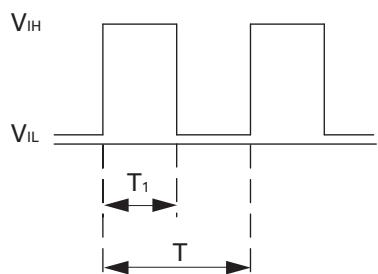
$$V_{IH} = 4.75 \text{ to } 5.25 \text{ V} \quad V_{IL} = 0 \text{ to } 0.4 \text{ V}$$
