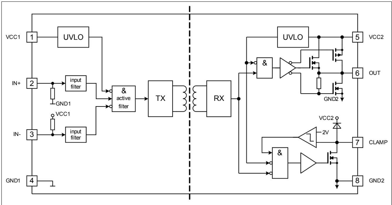
Figure 2 Block Diagram 1EDI10I12MF, 1EDI20I12MF and 1EDI30I12MF
