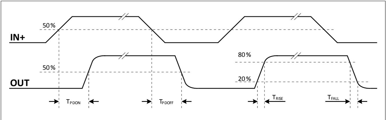
Figure 5 Propagation Delay, Rise and Fall Time
