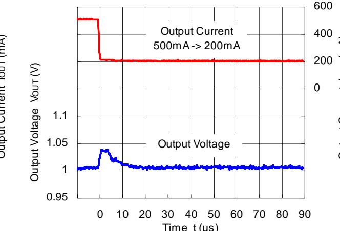
RP507K001B ( $V_{IN}=3.6V$ ,  $V_{OUT}=1.2V$ )
