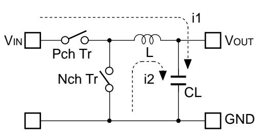
**Figure 1. Basic Circuit**
