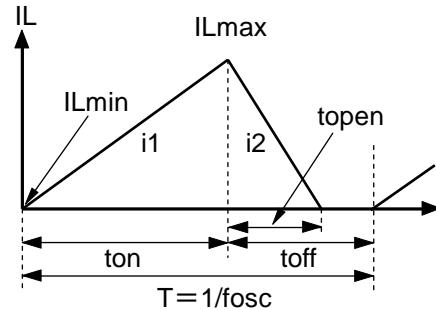
**Figure 2. Inductor Current ( $I_L$ ) flowing through Inductor**
