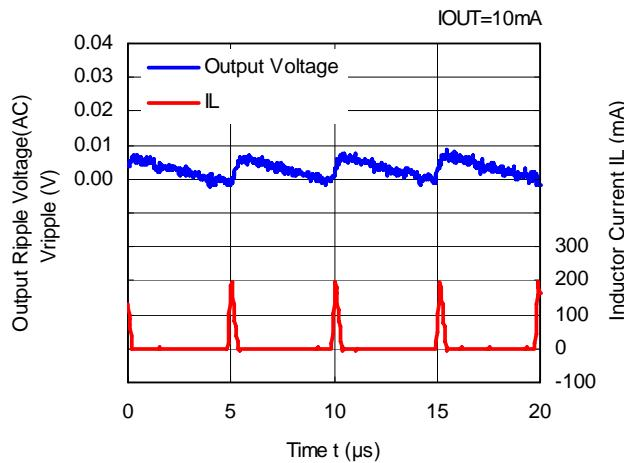
**RP507K001B V<sub>OUT</sub>=1.2V (V<sub>IN</sub>=3.6V)**
