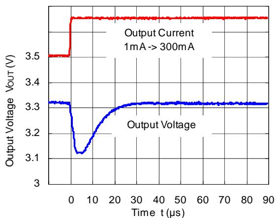
RP507K001B ( $V_{IN}=5.0V$ ,  $V_{OUT}=3.3V$ )
