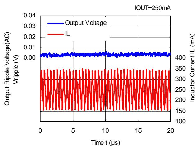
**RP507K001B V<sub>OUT</sub>=1.2V (V<sub>IN</sub>=3.6V)**
