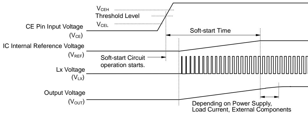
Soft-start time starts when soft-start circuit is activated, and ends when the reference voltage reaches the specified voltage.
