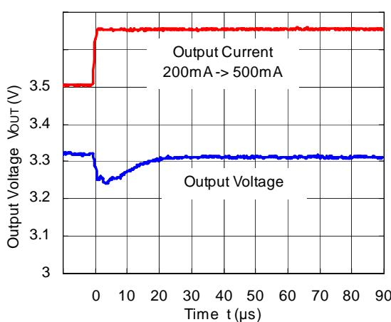
RP507K001B ( $V_{IN}=5.0V$ ,  $V_{OUT}=3.3V$ )
