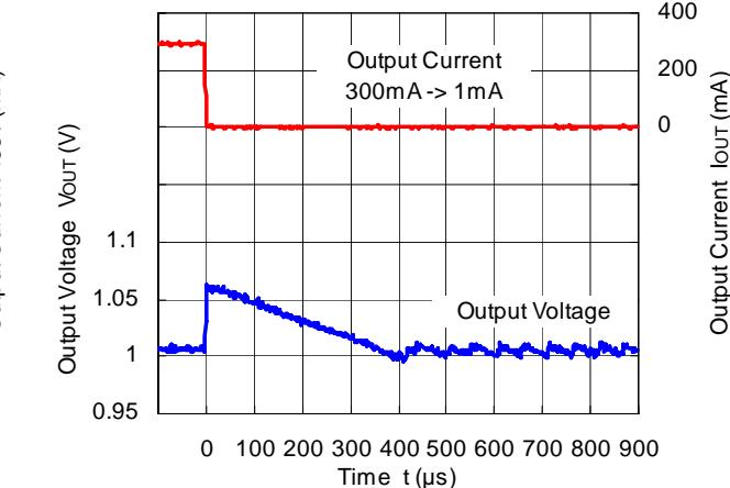
RP507K001B ( $V_{IN}=3.6V$ ,  $V_{OUT}=1.0V$ )
