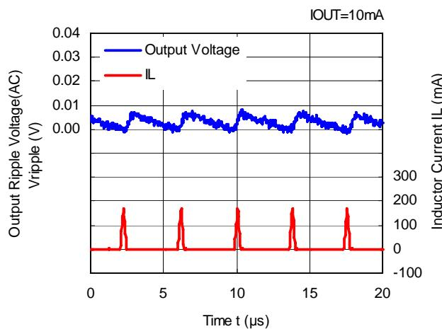
**RP507K001B V<sub>OUT</sub>=1.8V (V<sub>IN</sub>=3.6V)**
