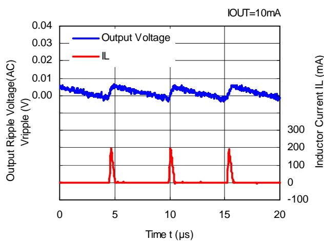
**RP507K001B V<sub>OUT</sub>=1.0V (V<sub>IN</sub>=3.6V)**
