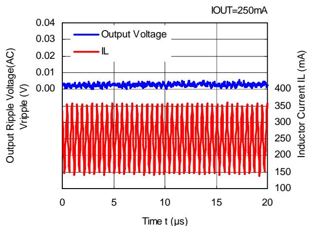
**RP507K001B V<sub>OUT</sub>=3.3V (V<sub>IN</sub>=4.3V)**
