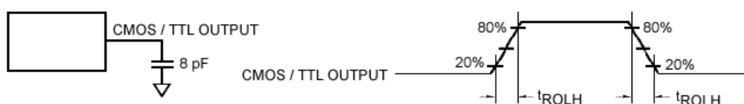
Figure 9. Receiver LVTTL/CMOS Output Load and Transition Times
