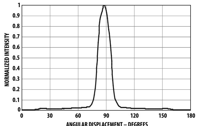
**Figure 8: Representative Spatial Radiation Pattern for 23° Viewing Angle Lamps**
