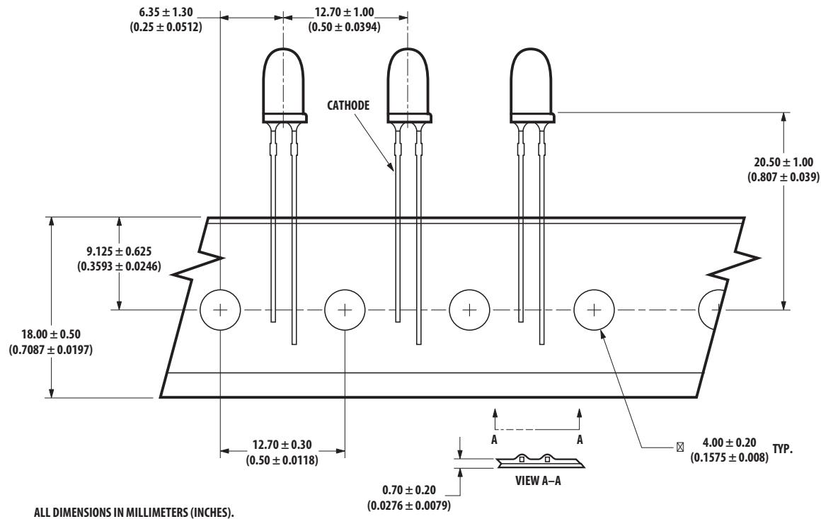
NOTE: THE AMMO-PACKS DRAWING IS APPLICABLE FOR PACKAGING OPTION -DD & -ZZ AND REGARDLESS OF STANDOFF OR NON-STANDOFF.
