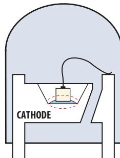
**NOTE:** Electrical connection between the bottom surface of the LED die and the lead frame is achieved through conductive paste.
