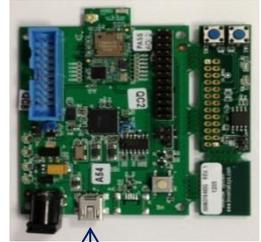
The ISM43362-M3G-EVB connects to the PC with a USB cable. The USB interface provides +5V power as well as individual programming and UART interfaces to the STM32F205 host processor (on the ISM43362-M3G-L44 module).
