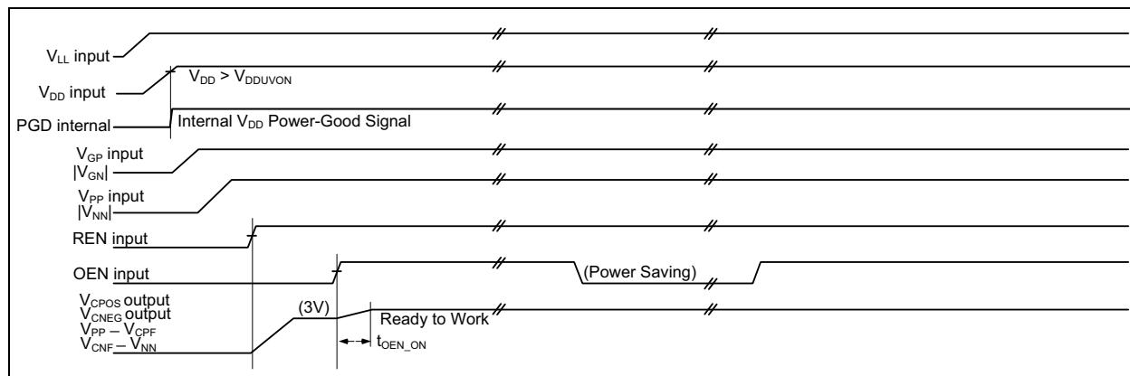
**FIGURE 4-1:** Power-On Events and Power-Saving Time Diagram.
