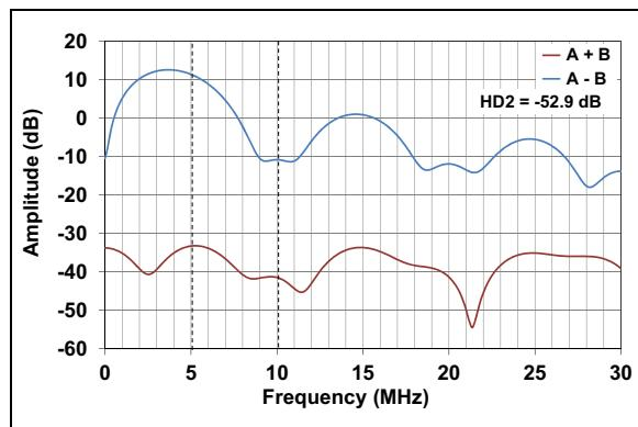
**FIGURE 2-8:** TX Output HD2, 1-Cycle
