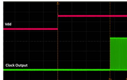
Figure 17. Startup Waveform vs. Vdd
