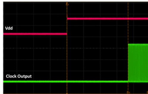
Figure 17. Startup Waveform vs. Vdd
