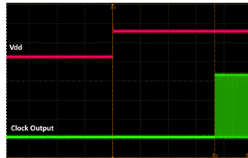
Figure 17. Startup Waveform vs. Vdd
