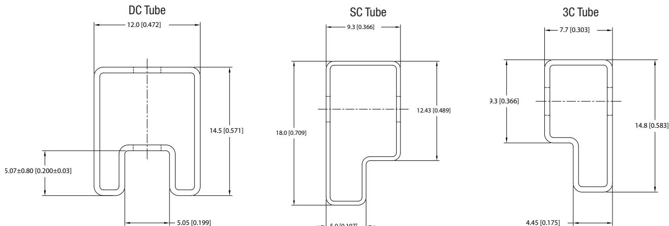
Unless otherwise specified all dimensions in mm [inches]  $\pm 0.55\text{mm}$  [0.022].
