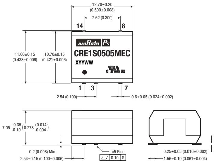
All dimensions in mm (inches) Controlling dimension is mm.
