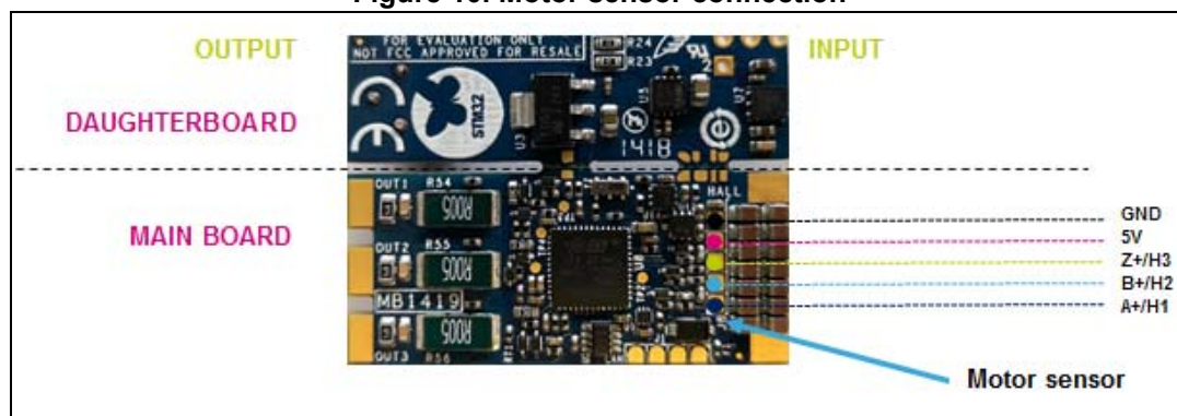
Figure 10. Motor sensor connection
