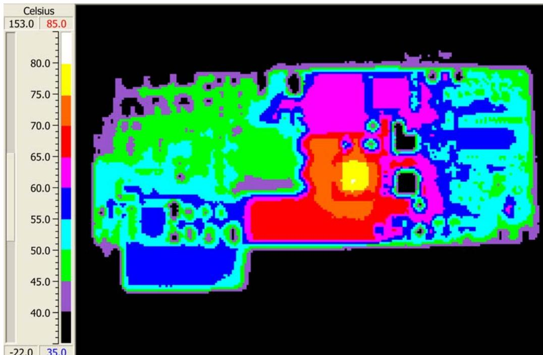
Figure 6. Thermal Map, Backside at  $48V_{IN}$  and  $11A_{OUT}$  ( $T_A = 25^\circ C$ , 200LFM)
