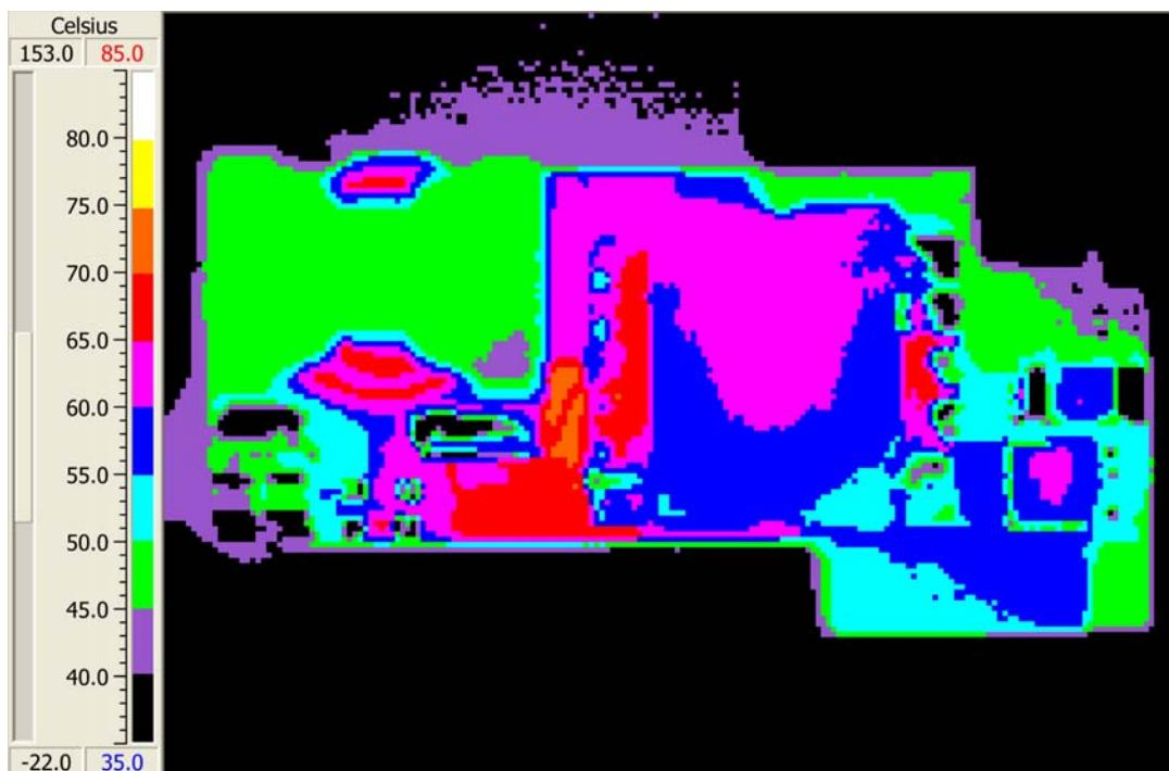
Figure 5. Thermal Map, Frontside at  $48V_{IN}$  and  $11A_{OUT}$  ( $T_A = 25^\circ C$ , 200LFM)
