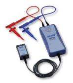
Low cost active differential probes are intended for measuring higher voltages. The differential techniques employed permit measurements to be taken at two points in a circuit without reference to the ground, allowing the oscilloscope to be safely grounded without the use of opto-isolators or isolating transformers.
