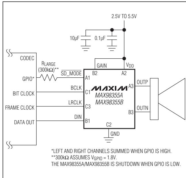
Figure 19. (Left + Right)/2 PCM Operation with 6dB Gain
