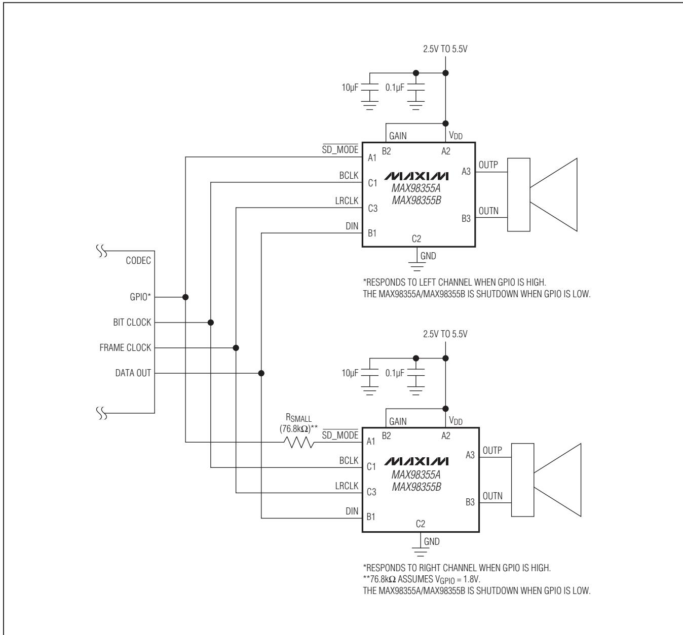
Figure 18. Stereo PCM Operation Using Two ICs
