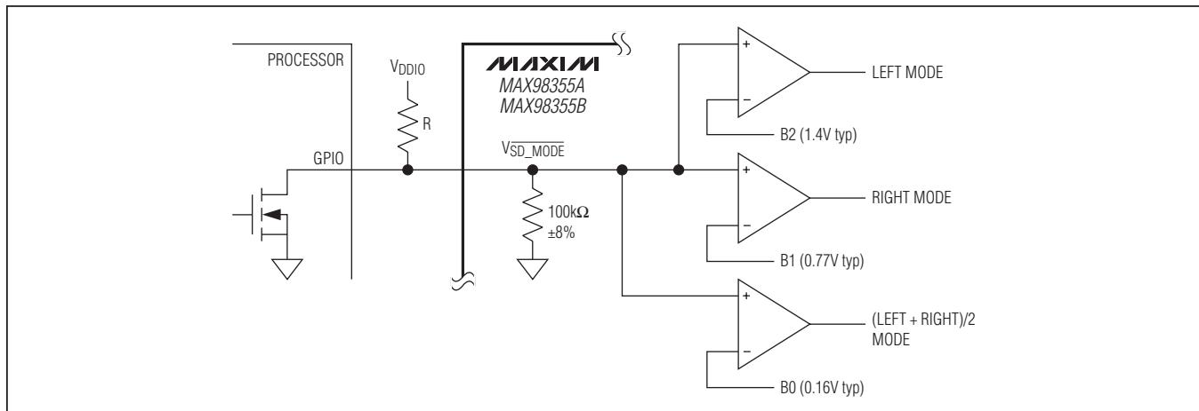
Figure 12. SD\_MODE Resistor Connection Using Open-Drain Driver
