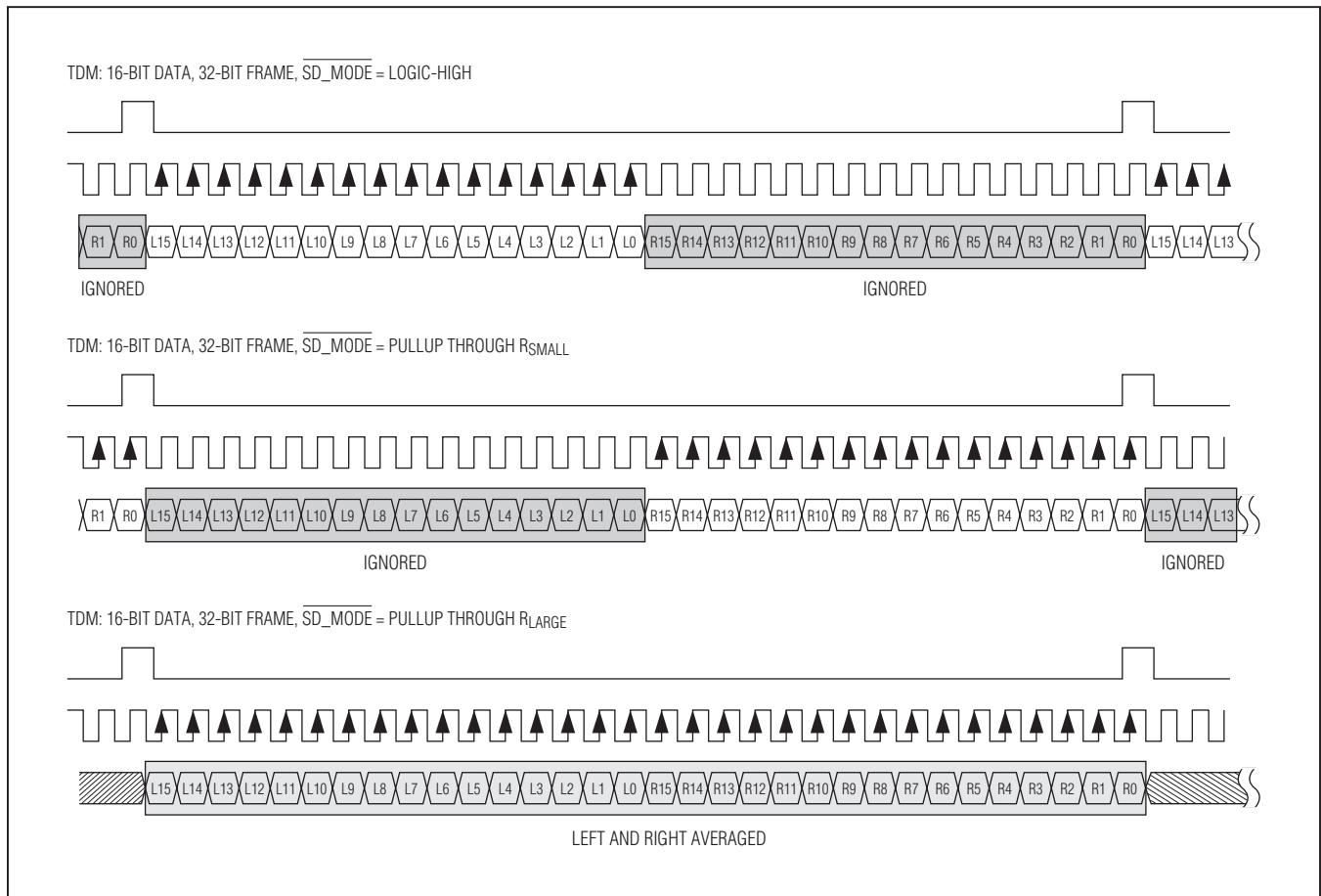
*Figure 8. MAX98355A TDM Digital Audio Interface Timing*
