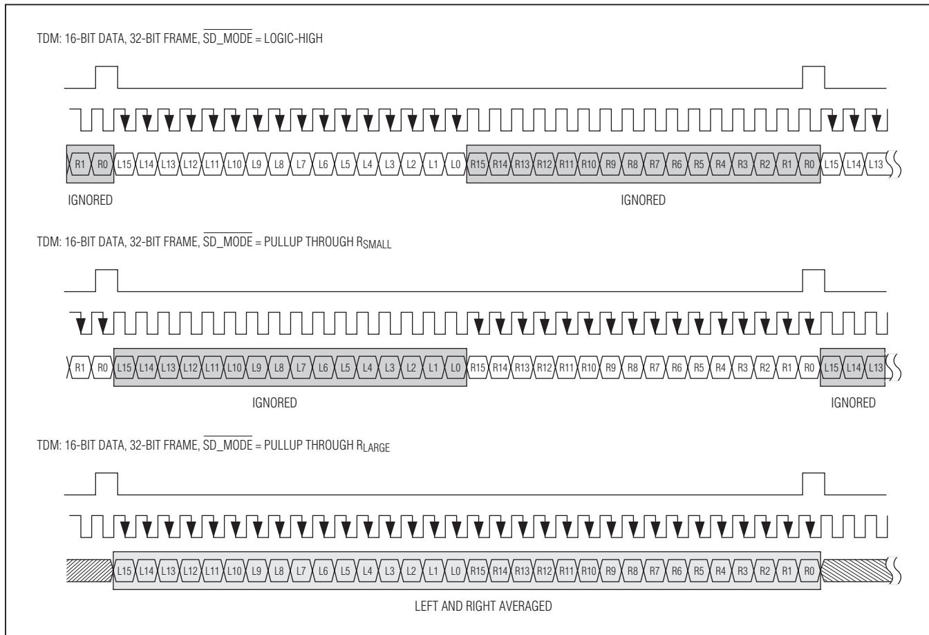
Figure 9. MAX98355B TDM Digital Audio Interface Timing
