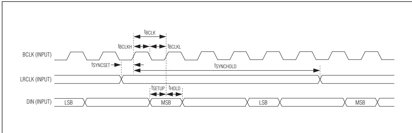
Figure 1. I<sup>2</sup>S Audio Interface Timing Diagram (MAX98355A)
