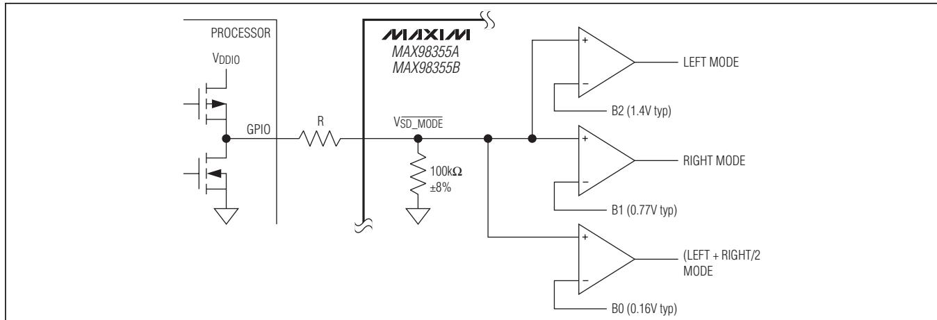
Figure 13. SD\_MODE Resistor Connection Using Pullup/Down Driver
