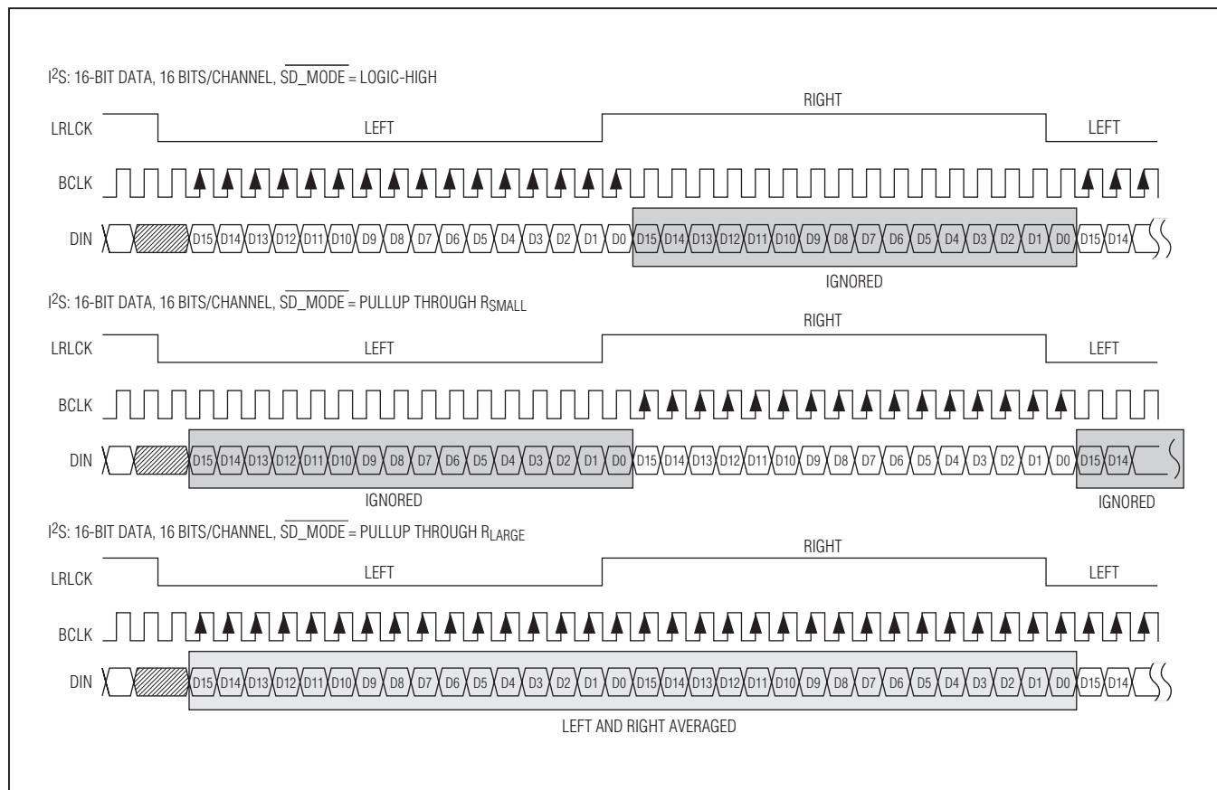
Figure 4. MAX98355A I<sup>2</sup>S Digital Audio Interface Timing, 16-Bit Resolution
