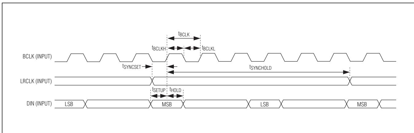
Figure 2. Left-Justified Audio Interface Timing Diagram (MAX98355B)
