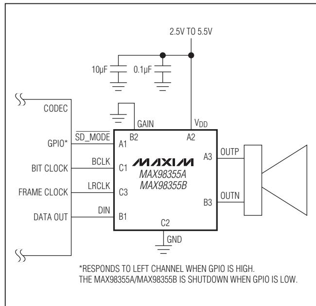
Figure 16. Left-Channel PCM Operation with 12dB Gain
