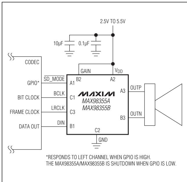
Figure 15. Left-Channel PCM Operation with 6dB Gain
